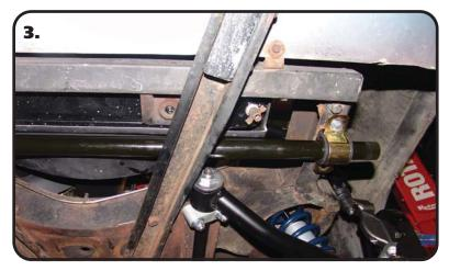
**3.** Insert the sway bar into position by sliding it between the bumper support and the frame rail. See **Step 1** for correct orientation. With the sway bar slid in place, install the mount bushing onto each end of the sway bar followed by the mounting strap.
