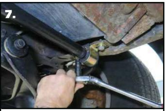
7. Again, the mounting holes need to be closest to the bend off the sway bar.. Install a 5/16" Lock Washer & 5/16" Flat Washer on (2) 5/16"x 1" Hex Bolts. Insert the hardware through the OEM swaybar mounting holes, threading the hardware in to the mount. Do NOT tighten the mounting hardware at this time.
