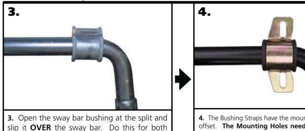
**4.** The Bushing Straps have the mounting holes that are offset. **The Mounting Holes need to be closest to the bend of the sway bar.** Slip the Bushing Straps over the Sway Bar Bushings.
