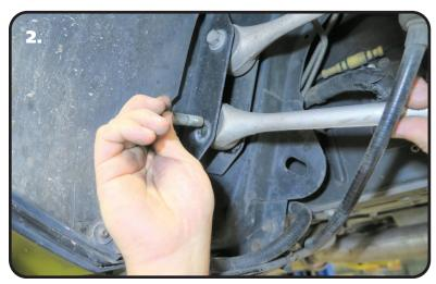
**2.** Start by removing the front mounting bolt for the lower trailing arm.
