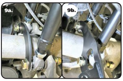
**9. Steps 10-13** cover attaching the rear of the R-Joint bars to the knuckle. If you are just upgrading the trailing arms to the R-Joint arms, the **"C" shaped tie plate (Image 9a)** supplied with the trailing arms will be used in the following steps. If you are installing Ridetech CoilOvers along with the trailing arms, the **lower CoilOver mount assembly (Image 9b)** will be installed during the installation of the trailing arms. Both brackets are shaped for clearance of the half shaft.
