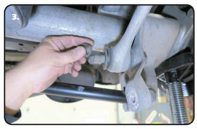
3. Remove the mounting hardware for the rear lower trailing arm. Retain the OEM washers that are on each side of the trailing arm bushings, they will be reused during the installation of the new trailing arm. The nut and bolt will be replaced with new ones that are included in the kit.
