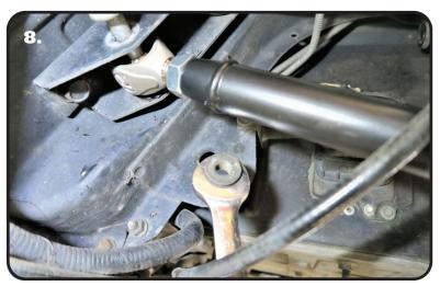
**8.** Install a 1/2" flat washer on the threads of the bolt. Put a 1/2"-13 nylok nut in the open end of a 3/4" wrench. You need to use the open end to be able to get the wrench out after installing the nut. Hold the nut in position with the wrench while threading the bolt into the nut. Torque the hardware to 63 ftlbs.
