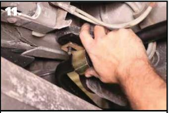
**11.** Install the bushing spacers under the swaybar bushings. They need to be installed with the bolt holes offest towards the wheel. The spacers will slide over the OEM mounting studs.
