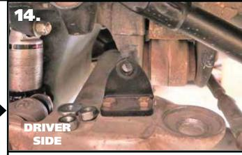
**14.** Install the new linkage mounts in place of the OEM mounts. They are installed with the mounting holes to the wheel. Line up the mounting holes with the OEM holes. Install a 5/16"-18 x 1 1/4" bolt, flat washer, and 5/16"-18 nylok nut. Torque hardware to 25 ftlbs
