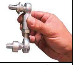
**16.** Install a T-bushing on one end of the linkage (small diameter out), with a .300" thick spacer on the other end. The end with the T-bushing will be the TOP end of the linkage that will be installed in the swaybar end.
