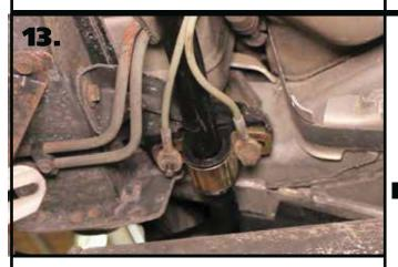
**13.** Use the OEM hardware to reattach the gas tank safety cables to the swaybar mounting studs.
