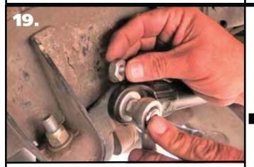
**19.** Install a M10-1.5 serrated lock nut on the threads of the upper stud of the linkage.
