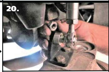
**20.** Install a M10 flat washer and M10-1.5 serrated lock nut on the threads of the lower stud of the linkage. Repeat Steps 15-20 on the other side. Torque the hardware to 37 ftlbs.
