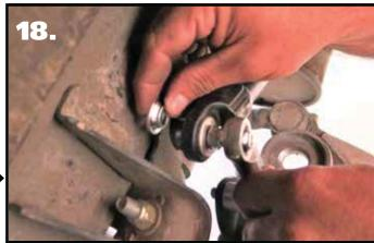
**18.** Install a 2nd T-bushing on the threads of the upper stud with the small diameter sticking into the swaybar end.
