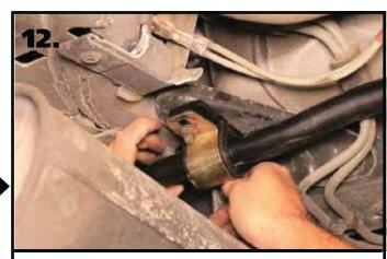
**12.** The swaybar bushings/straps will slip in place on the OEM studs. Push the swaybar up inplace. Reuse the OEM hardware to attach the swaybar bushings/swaybar to the car. Torque nuts to 18 ftlbs.
