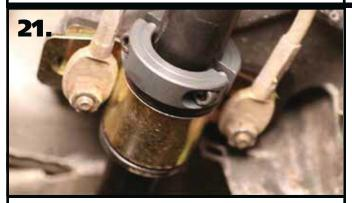
**21.** Disassemble the Locking Rings provided in the kit. The locking rings will need to be installed against the inside edge of the swaybar bushings. Assemble each locking ring against the swaybar bushing and tighten.
