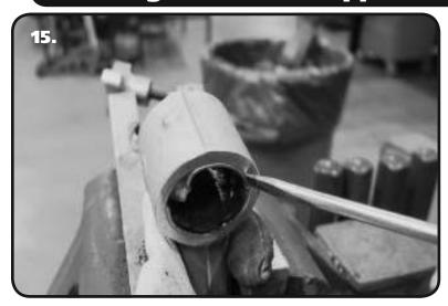
**15.** Using a smaller chisel and hammer to fold the inner side of the bushing inward. Again, do this on the same 1/2 of the bushing as the previous step. The bushing will start coming out as you bend it inward.
