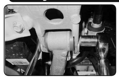
**25.** Tighten each Cam Nut, but first align the mark made on the Cam. Hold the Adjusting Cam Bolt Head in place with a wrench while torquing the Cam nut. Torque the Cam Nut to 125 ftlbs.
