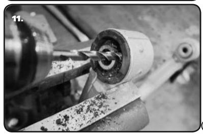
**11.** Using a drill and 5/16" drill bit, drill the rubber out of the bushing. You can start by plunging several holes around the bushings. Drill as many holes as you can leaving very little rubber. The remaining rubber can be cut out with the drill bit by going in a circular motion around the inner sleeve. Let the drill do the work for you. Remove the inner sleeve when it comes loose.
