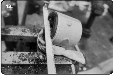
**13.** Cut through the outer flange of the bushing in line with the 2 cuts made on the inner ID. Try to avoid cutting into the arm.
