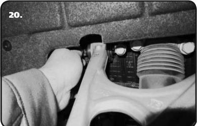
**20.** Reinstall the Control Arm on the car with any shims back into their previous location. Tighten all Fasteners.
