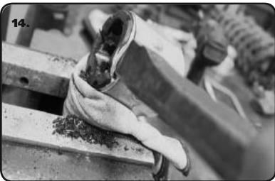
**14.** Using a Hammer and Chisel, bend in the outer flange beside one of the cuts. Bent it enough to distort the ID of the bushing. We found bending in the flange beside both cuts on the same 1/2 of the cut bushing sleeve worked the best.
