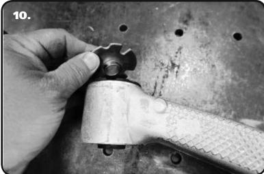
**10.** Remove the large T-bushing from the outer side of the OEM bushing. This can be done by simply prying them out with a small pry bar.
