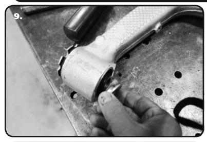
**9.** Remove the small T-bushing from the inner side of the OEM bushing. This can be done by simply prying them out with a small pry bar.
