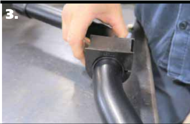
3. Open the sway bar bushing at the split and slide it OVER the swasy bar. Do this for both bushings.
