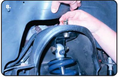
**8.** Install a 7/16" flat washer on each of (3) 7/16"-14 x 1 3/4" hex bolts. Align the mounting holes of the upper mount with the mounting holes in the frame. The mounting bolts need to be installed with the threads pointing up. Insert a bolt/washer in each holes. Install a 7/16" flat washer and 7/16"-14 nylok nut on the threads of each bolt sticking through the frame. Torque the hardware to 50 ftlbs.
