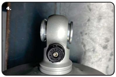
**4.** Install the 1/2" I.D. bearing spacers into the bearing in the shock eyelet. These spacers have a through hole that is 1/2" diameter. The small side of the spacers will insert into the shock bearing.
