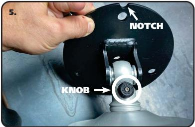
5. Attach the upper mount to the shock eye. The mount needs to be attached to the eyelet so that the notch is on the same side as the adjuster knob.
