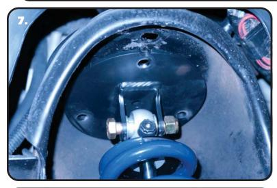
**7.** Put the ShockWave in position on the truck. The upper mount needs to be positioned with the NOTCH toward the wheel. The shock adjuster knob should also be toward the wheel.
