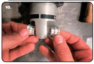
**10.** Install the 1/2" I.D. bearing spacers into bearing in the shock body. These spacers have a through hole that is 1/2" diameter. The small side of the spacers will insert into the shock bearing.
