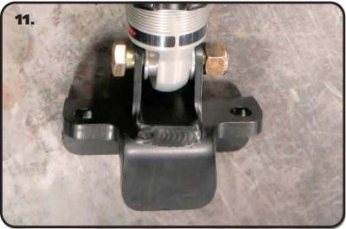
**11.** Insert the shock into the Lower Mount. Line up the shock bearing/spacers hole with the mounting holes of the lower mount. Insert a 1/2"-13 x 2 3/4" bolt through the mount/ shock. Install a 1/2" flat washer and 1/2"-13 nylok nut on the threads of the bolt that are sticking through the mount.
