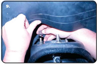
**9.** Slide the wire loom clip on the threads of the front upper mounting bolt.
