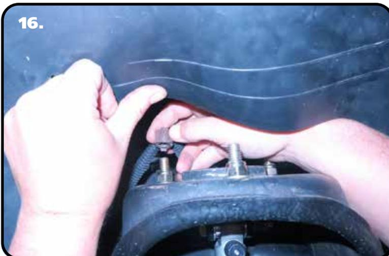
**16.** Slide the wire loom clip on the threads of the front upper mounting bolt.
