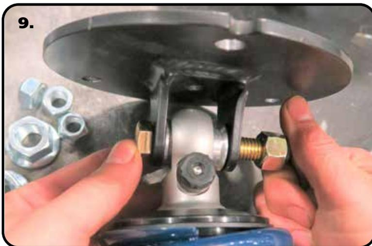
9. Insert the shock eyelet into the Upper Mount. Line up the shock bearing/spacers hole with the mounting holes of the upper mount. Insert a 1/2"-13 x 2 3/4" bolt through the mount/shock. Install a 1/2" flat washer and 1/2"-13 nylok nut on the threads of the bolt that are sticking through the mount. Torque the upper and lower mounting hardware to 75 ftlbs.
