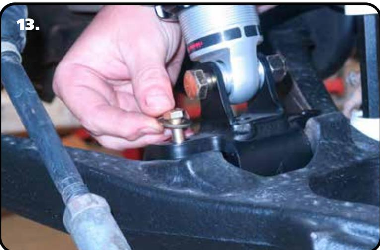
**13.** Align the mounting holes of the lower mount with the OEM shock mounting holes in the lower control arm. Install a 3/8" flat washer on each of (2) 3/8"-16 x 2 1/4" hex bolts. Insert the bolts/washers in the aligned holes of the lower mount and control arm.
