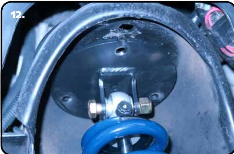
**12.** The Upper Mount needs to be positioned with the NOTCH toward the wheel. The shock adjuster knob should also be toward the wheel.
