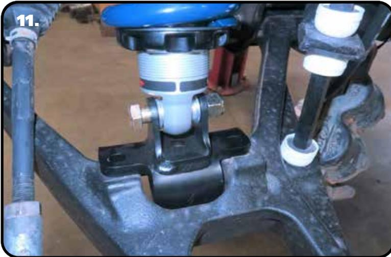
**11.** Put the CoilOver in position on the truck. The Lower Mount will only attach to the control arm one way. The SMALL vertical tab needs to be positioned toward the wheel.
