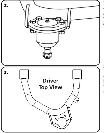
**2.** Install the ball joints into the upper control arm with the hardware supplied with the ball joint. The upper ball joint goes in from the top side of the control arm. The gussets on the ball joint plate point up. Torque the hardware to 18 ftlbs.
