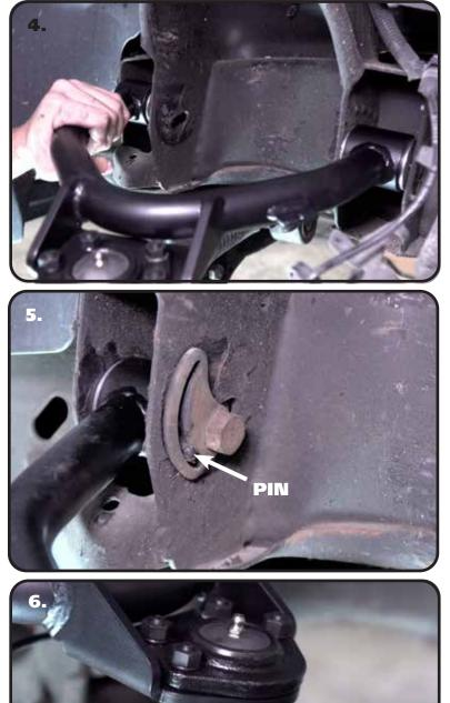
**4.** The upper control arm is attached in the factory mount using factory hardware. The driver side arm is shown in **Figure "3 & 4"**. Line up the through holes of the bushings with the OEM slots.
