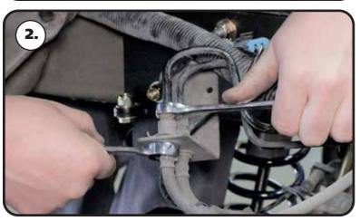
**2.** The brake line bracket that bolted to the top of the driver frame rail will need to be replaced with one supplied in the kit. Start by loosening the lines using line wrenches.
