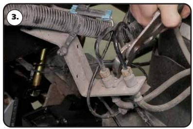
**3.** Remove the clips that hold the brake lines in place. Retain the clips for installation of the new bracket.
