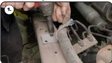
**1.** Unbolt the brake line bracket from the top of the driver frame rail. We have the bed off for this photo to better show the bracket and hardware. You do NOT have to remove your bed to install this kit.
