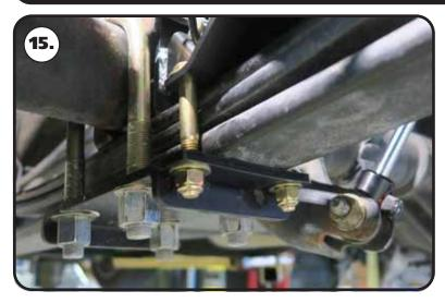
**15.** Slip the spring clamping plate on the threads of the 2 bolts sticking down past the leaf spring. Install a 7/16" flat washer & 7/16"-14 nylok nut on each bolt. Tighten the hardware to 50 ft-lbs.
