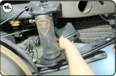
**16.** The inner frame plate is side specific. THE DRIVER SIDE HAS A LARGE HOLE IN THE BRACKET. The passenger side does NOT have a hole.
