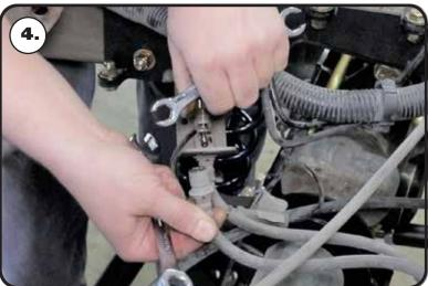
**4.** Separate the lines and remove them from the bracket. Thread the lines back together and tighten them using line wrenches. The new bracket has slots for the lines to slip through.
