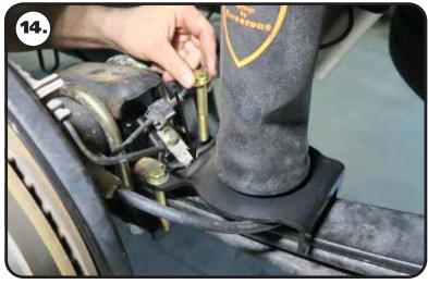
**14.** Install a 7/16" flat washer on each of (2) 7/16"- 14 x 3" bolts. Insert the bolts/washers in the forward 2 holes of the lower bracket.
