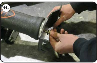
**11.** Attach the lower air spring mount to the bottom of the air spring using red loctite, a 3/8"-16 x 1" bolt & 3/8" SAE flat washer. DO NOT TIGHTEN AT THIS TIME.
