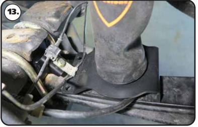
**13.** Use Images 13-15 as a reference for attaching the lower air spring bracket. The bolt holes need to be toward the axle with the forward "hook" hooking the u-bolt. The "hook" will help with positioning of the lower mount. The rear of the mount has 2 tabs that will sit on each side of the leaf spring. The emergency brake cable will run UNDER the bracket.
