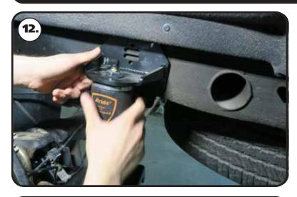
**12.** Put the air spring assembly in place on the leaf spring BEHIND the differential. The narrow part of the upper air spring mount will go to the front of the truck.
