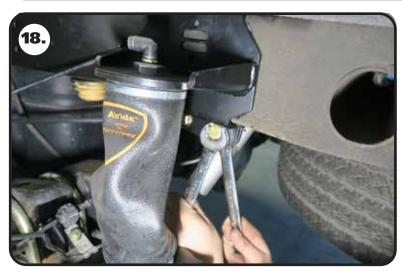
**18.** Install a 1/2" flat washer on each of (4) 1/2"-13 x 1 3/4" hex bolts. Insert them through the aligned holes of the air spring mount and inner plate. Install a 1/2" flat washer and 1/3"-13 nylok nut on the threads of the bolts. Push the upper mount to the rear of the truck, making sure it is tight on the frame. Torque to 75 ft-lbs.
