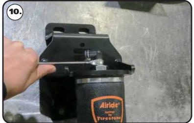
**10.** Put thread sealant on the 90 degree air fittings and thread them into the top of each air spring and tighten. Proper tighten of a pipe thread is, finger tight plus 1 1/2 turns with a wrench.
