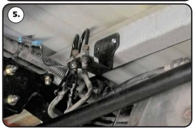
**5.** Slip the brake line(s) into the new bracket and reinstall the clips. Screw the brake line bracket to the bed brace using the supplied #10 x 3/4" self drilling screws.
