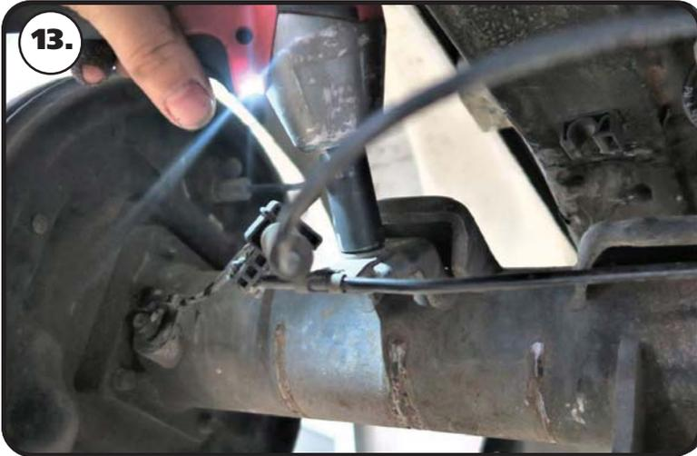
**13.** Remove the bolt from the brake line retainer. The brake line retainer bolts to the bracket that is on the rear side of the leaf spring perch. Remove these from both sides of the axle. These will be reinstalled later.
