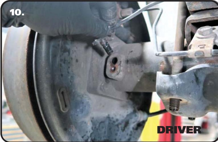
**10.** Remove the ABS sensors from the axle tubes on driver and passenger side. **DRIVER SIDE IS SHOWN IN IMAGE 10.**
