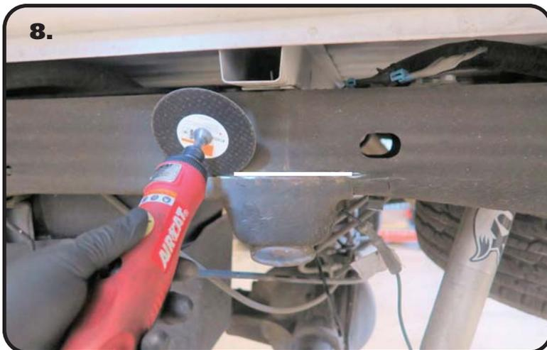
8. The OEM bump stop mount will need to be cut off the frame. We do this by cutting the weld with a cut off wheel on a die-grinder. Cut in the center of the weld without going too deep. Cutting too deep will cut into the frame.
