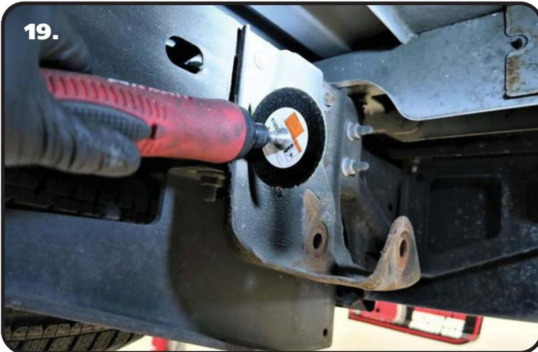
**19.** The rear leaf spring hanger will need to be removed from the frame. It is held on by (1) bolt and (3) rivets. Remove the bolt and retain it for installation of the new hanger. We remove the rivets by cutting a " + " in the rivet head and chiseling it off. After chiseling the head off, drive the rivet out of the hanger/frame with a punch.
