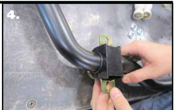
4. Slip the Bushing Straps over the SwayBar Bushings.
