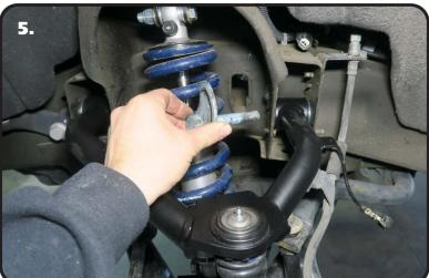
**5.** The upper control arm is attached in the factory mount using factory hardware. The driver side arm is shown in **Figure "3, 4 & 5"**. Line up the through holes of the bushings with the OEM holes.
