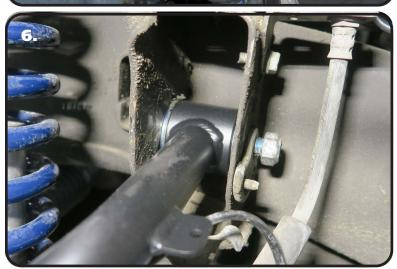
**6.** Reinstall the OEM bolts. Snug the hardware down for now. The upper control arm bolts need to be torqued to 140 ft-lbs.
