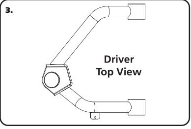
**3.** The upper control arm is attached to the factory mount using the factory hardware. The driver side arm is shown in **Figure "3"**. The ball joint on the arm is oriented to the rear of the truck. The brake line tab on the control arm will be to the RFAR of the control arm.
