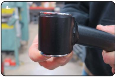
**4.** Insert a t-washer in each side of the control arm bushings. The small diameter of the t-washer goes into the bushing. You may have to tap it in the inner sleeve. The control arm mount will keep the t-washer seated.
