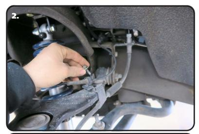
**2.** Remove the brake line tab from the upper arm.
