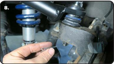
**8.** Install the ball joint nut on the ball joint pin.
