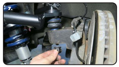
**7.** Insert the pin of the upper ball joint into the spindle.
