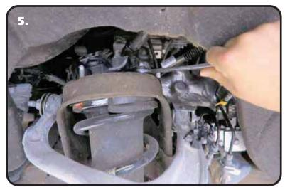
**5.** With the suspension supported with a jack, remove the 3 upper shock/spring retaining nuts.
