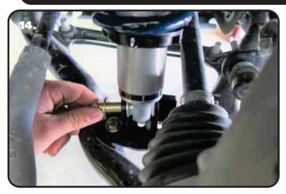
**14.** Insert the small diameter of the aluminum shock spacers into each side of the shock bearing in the shock body. Insert the shock body into the lower mount. Line up the shock bearing/spacers hole with the mounting holes of the lower mount. Insert a 1/2"-13 x 2 3/4" bolt through the mount/shock.
