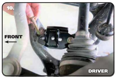
**10.** Align the lower mount with the OEM shock mounting holes. The mount needs to be positioned with the bent tab to the inside of the truck. The shock mounting tabs need to be offset to the front of the truck. Install a 7/16" flat washer on each of (2) 7/16"-14 x 2 1/4" bolts. Insert the bolt/washers through the mount and control arm. Install a 7/16" flat washer and 7/16"-14 nylok nut on the threads of each bolt. Torque to 70 ft-lbs.
