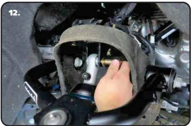
**12.** Insert the shock eyelet into the upper mount. Line up the shock bearing/spacers hole with the mounting holes of the upper mount. Insert a 1/2"-13 x 2 3/4" bolt through the mount/shock. **MAKE SURE THE ADJUSTMENT KNOB IS FACING OUT TO THE WHEEL.**
