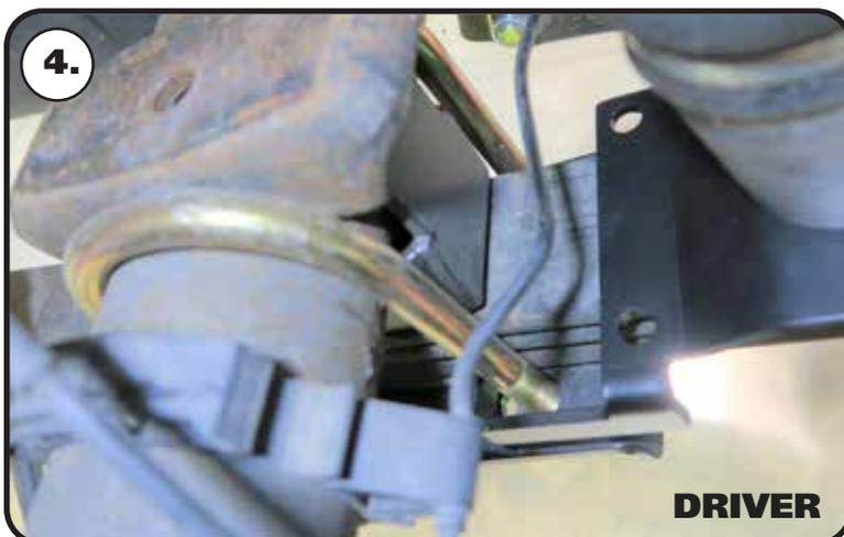
4. Use Images 4-6 as a reference for attaching the lower air spring bracket. The bolt holes need to be toward the axle with the forward "hook" hooking the u-bolt. The "hook" will help with positioning of the lower mount. The rear of the mount has 2 tabs that will sit on each side of the leaf spring.
