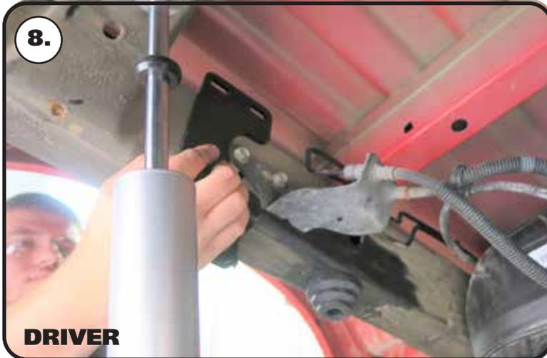
**8.** Hold the inner plate in position. It is bent to wrap under the frame rail. The (4) bolt holes will line up with the bolt holes of the upper air spring mount.
