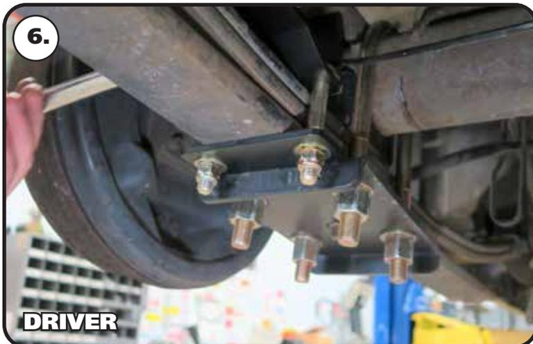
6. Slip the spring clamping plate on the threads of the 2 bolts sticking down past the leaf spring. Install a 7/16" flat washer & 7/16"-14 nylok nut on each bolt. Tighten the hardware to 50 ft-lbs.
