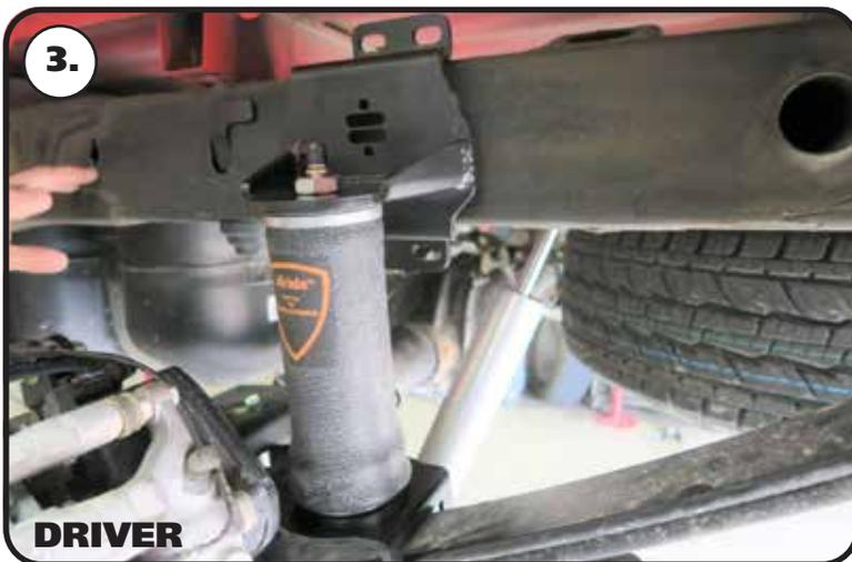
3. Put the air spring assembly in place on the leaf spring BEHIND the differential.
