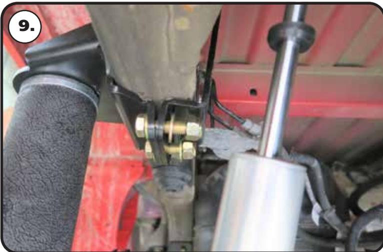
**9.** Install a 1/2" flat washer on each of (4) 1/2"-13 x 1 3/4" hex bolts. Insert them through the aligned holes of the air spring mount and inner plate. Install a 1/2" flat washer and 1/3"-13 nylok nut on the threads of the bolts. Make sure the top and bottom air spring mounts are inline with each other. Torque to 75 ft-lbs.
