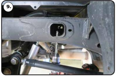
**9.** The 1/2" hole needs to drilled through the bottom of the crossmember too.
