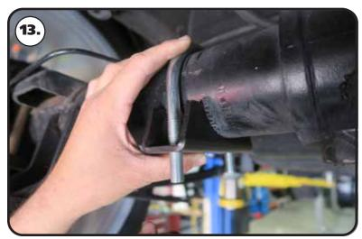
**13.** Slip the axle mount onto the u-bolts. The "teeth" of the axle bracket will sit against the axle tube.
