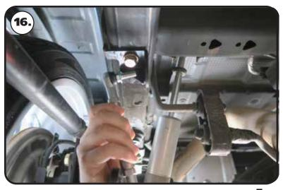
**16.** Install a M10 flat washer on the threads of the PosiLink. Insert the PosiLink in the mounting hole of the frame bracket with the threads of the end link pointing to the center of the truck.
