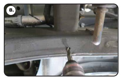
**8.** Drill the bottom of the frame with a 1/2" drill bit.
