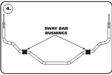
**4.** Open the sway bar bushing at the split and slip it **OVER** the sway bar at the locations shown in *Image 4*. Do this for both bushings.
