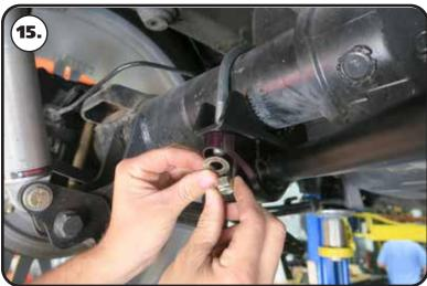
**15.** Install a 7/16" flat washer & 7/16"-20 nylok nut on the threads of the u-bolts. Center the sway bar on the axle. Snug the hardware down and verify the axle mounts are parallel with the leaf springs. Torque the u-bolt hardware to 35 ft-lbs.
