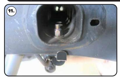
**11.** Install a 1/2" flat washer & 1/2"-13 nylok nut on the threads of the bolt sticking into the crossmember. Torque to 75 ft-lbs. Repeat the previous steps for the frame bracket on the other side.
