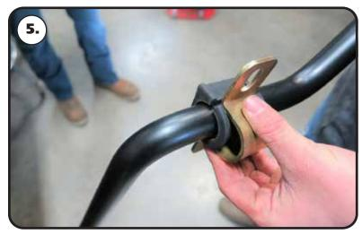
**5.** Install the bushing straps over the sway bar bushings.
