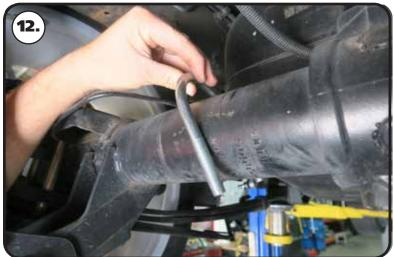
12. Install a 7/16" u-bolt on each axle tube
