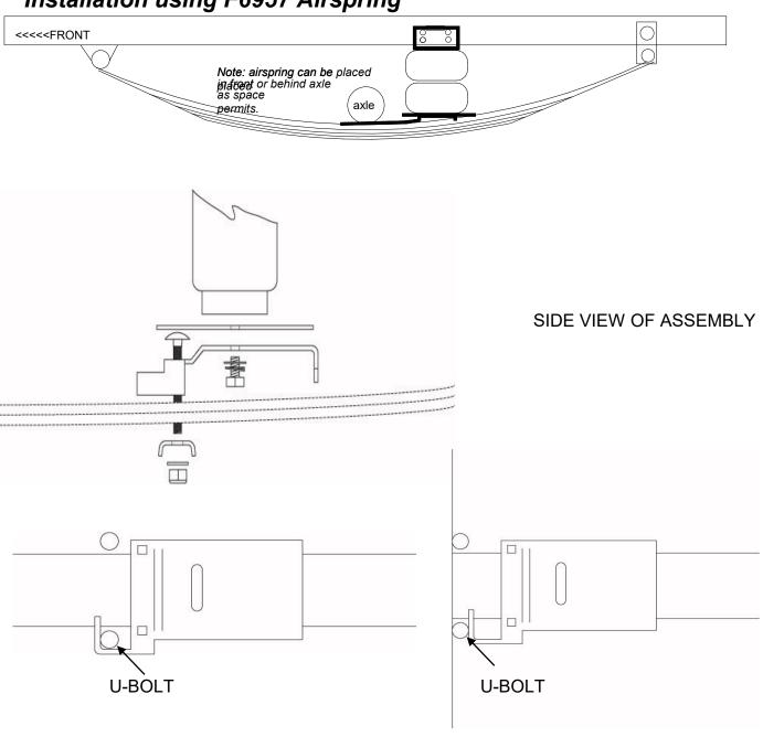
THE LEAF SPRING BRACKET CAN BE INSTALLED HOOKED ON THE U-BOLT OR TOUCHING U-BOLT AS SEEN IN ABOVE ILLUSTRATIONS.
