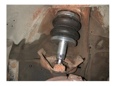
1. The ShockWaves will be installed in place of the OEM coil spring and shock assembly using the OEM shock mounting points as shown in the picture below.
