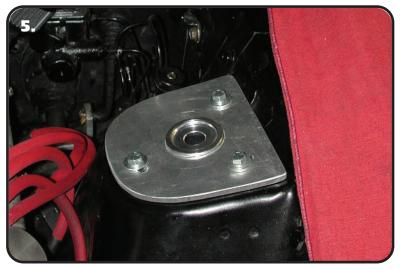
**5.** Lay the Upper Plate on Top of the shock tower with the ShockWave Mount protruding through the large center hole. Line up the the holes in the Upper Plate with the holes drilled in the shock tower and the holes in the ShockWave mount. If the INNER Hole doe not line up, flip the plate over. Install a 5/16" x 1" Flange Bolt in each hole and tighten.
