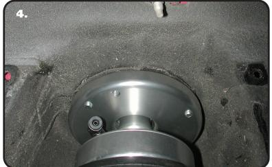
**4.** Hold the Aluminum Upper Mount agianst the bottom of the shock tower lining up the threaded holes with the holes drilled in the shock tower.
