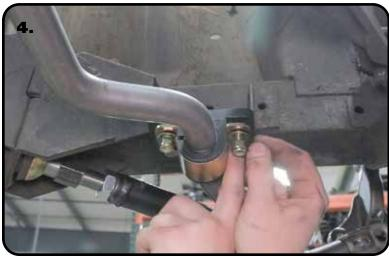
**4.** Slide the sway bar into position on the car. The sway bar arms will be bending upward with the center dropping toward the ground. Install a 3/8" flat washer on (4) 3/8"-16 x 1 1/4" hex bolts. A bolt/washer will go in each of the 4 mounting holes. With the bolt/washers installed, install a 3/8" flat washer on the threads followed by a 3/8"-16 nylok nut. Do **NOT** completely tighten the hardware. It will be left partially loose until the end links are installed.
