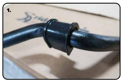
**1.** Open the sway bar bushing at the split and slip it **OVER** the sway bar. Do this for both bushings.
