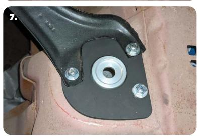
7. Install the export brace on the bolts sticking through the top plate. Install a 3/8" SAE flat washer & 3/8"-16 nylok nut on the threads of each of the bolts. Torque the nylok nuts to 15 ft-lbs.
