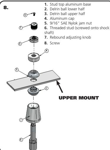
time. **8.** The air fitting location can be rotated by twisting the bellow assembly separate of the shock. Place the Shockwave into the coil spring pocket with the stud sticking through the OEM shock hole. See assembly **Diagram 8**.
