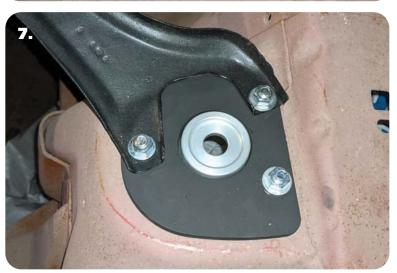
7. Install the export brace on the bolts sticking through the top plate. Install a 3/8" SAE flat washer 7 3/8"-16 nylok nut on the threads of each of the bolts. Torque the nylok nuts to 15 ft-lbs.
