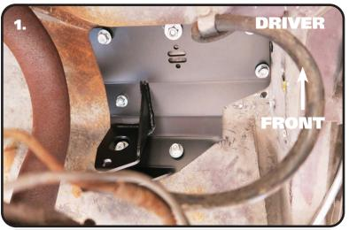
1. The Driver Upper Shock Mount repositions the top of the shock to behind the axle. The Mount nests in the car one way. Position the Mount in the car with the Shock attaching point to the rear and away from the frame. The outside edge of the mount will touch the frame with the front edge against a body seam. Using these points as a guide, the Mount will fit the contours of the body. With the Mount in position, use it to mark the 7 holes and drill them 5/16"
