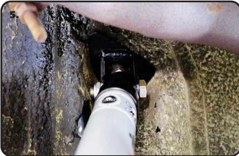
**5.** The Shock is mounted in the Upper Mount with the BODY UP. It is held in place with a 1/2"-20 x 2 1/4" Hex Bolt & 1/2"-20 Nylok. If the threads of the bolt would happen to touch the floor pan of the car, a 1/2" Flat Washer can be installed under the head of the bolt.
