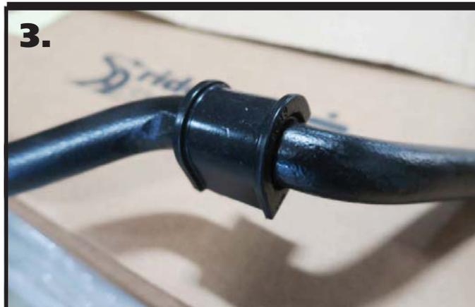
**3.** Open the sway bar bushing at the split and slip it **OVER** the sway bar. Do this for both bushings.
