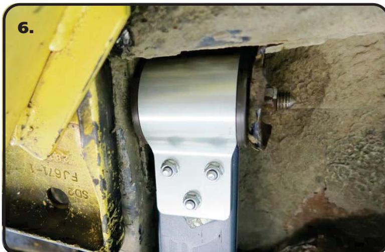
**6.** Swing the Leaf Spring up and attach the **LARGE BUSHING END** of the Composite Leaf Spring into the OEM front leaf spring mount using a 1/2"-13 x 4.5" Hex Bolt and 1/2"-13 Nylok Nut.
