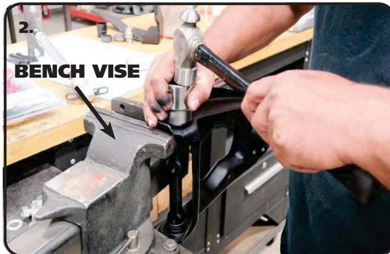
2. Disassemble the Bushing being installed. When installing Bushings in the control arms, insert the Cross Shaft before installing any Bushings. Support the back side of the flange the Bushing is being Installed in. They can be supported by either the piece of Metal or by the Bench Vise with the Jaws opened wide enough to let the Bushing Shell pass through (Image 2).
