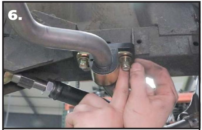
**6.** Install the sway bar in position in the car. The center of the bar should be to the front of the car. The outer arms of the sway bar will bend upward. Install a 3/8" flat washer on (4) 3/8"-16 x 1 1/4" hex bolts. A bolt/washer will go in each of the 4 mounting holes. With the bolt/washers installed, install a 3/8" flat washer on the threads followed by a 3/8"-16 nylok nut. Do **NOT** completely tighten the hardware. It will be left partially loose until the end links are installed.
