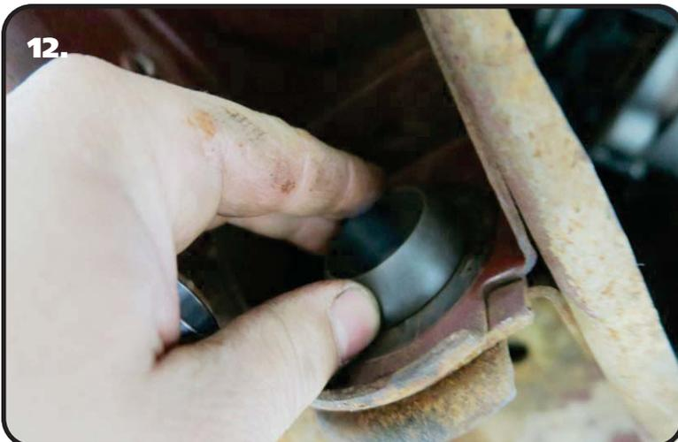
**11.** Refer to **(Image 14)** for the Delrin Strut Rod Bushing assembly order. The Delrin Strut Rod Bushing will insert into the frame bushing hole with the rounded side of the bushing outward. A Bushing needs to be installed on both the front and rear side of the frame.
