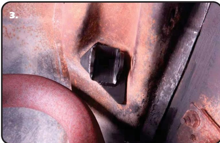
3. Install the Passenger Shock Mount will be installed in the OEM location. The Shock Mount is shaped to fit the body and will only fit into the OEM location one way. Install the mount into the OEM location with the Stud sticking through the OEM shock hole. Have someone hold the mount in place while installing the top support and mounting hardware,
