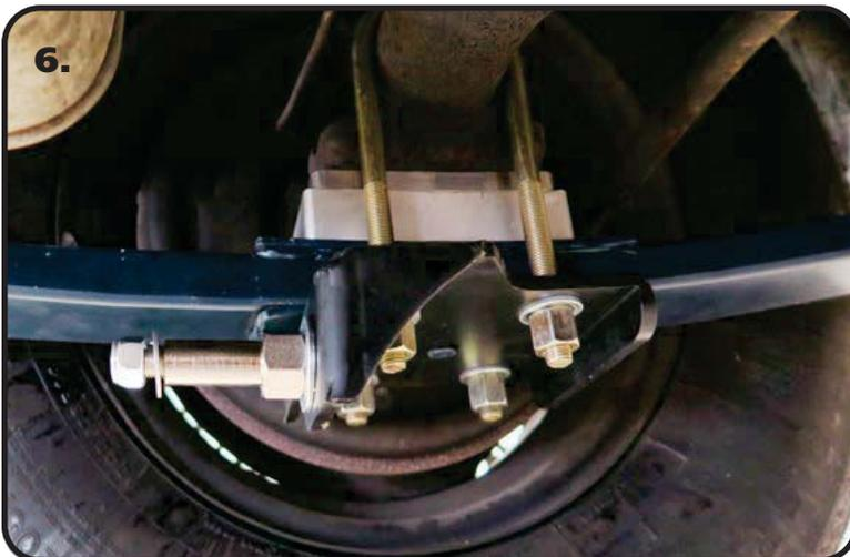
**6.** The Lower Shock is Bolted to the Lower Shock Mount using the supplied Shock Stud. Install the Studs into the Lower Mounts with a Washer on each side of the Mount. Slide a Washer onto the Stud. Jack the Rear Differential up until the Shocks can be slid onto the Shock Stud. Slide the Shock onto the Stud with the Adjuster Knob pointing inward. Install the supplied 7/16" Flat Washer and Nylok Nut onto the Threads and tighten.
