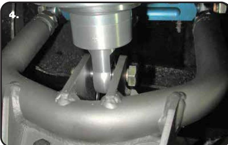
4. Attach the Shockwave to the upper StrongArm using a  $\frac{1}{2}$ " x  $2\frac{1}{4}$ " bolt and Nylok nut. Torque to 75 ft-lbs.
