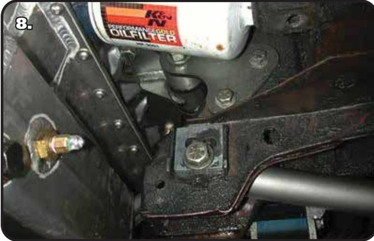
**8.** Eccentric eliminator plates are included, one must be installed on each side of the frame. Start out with it in the center, make sure both plates are in the same position. Attach the other end of the lower control arm to the factory frame mount using a 1/2" x 4 1/2" bolt and Hex nut. Torque to 75 ft-lbs.
