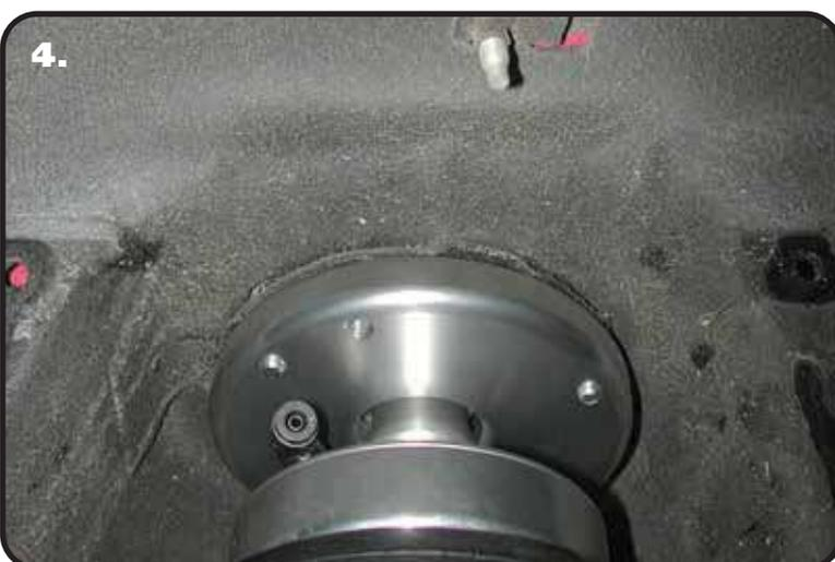
4. Hold the aluminum upper mount against the bottom of the shock tower lining up the threaded holes with the holes drilled out in the shock tower.
