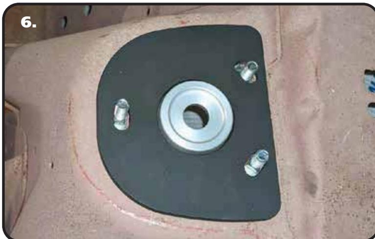
6. Lay the upper plate on top of the shock tower with the ShockWave mount protruding through the large center hole.
