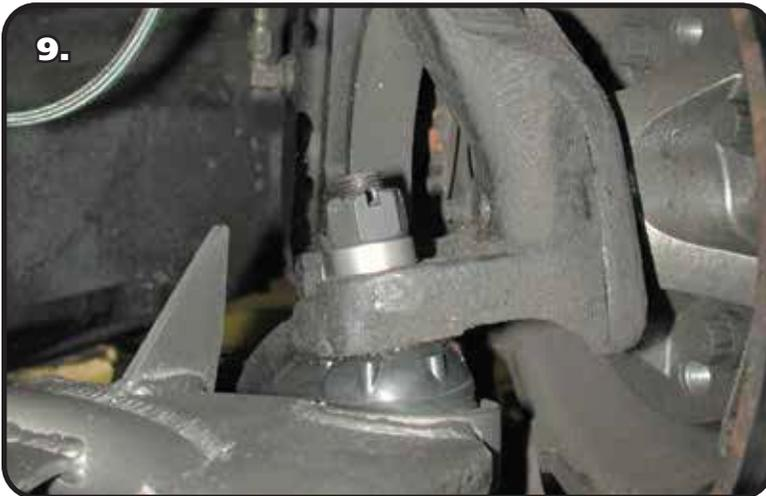
**9.** Slide the ball joint boot over the ball joint, then place the spindle over the ball joint stud. A ball joint spacer will be necessary to align the castle nut with the cotter pin hole. Grease ball joint. Attach the spindle to the control arms.
