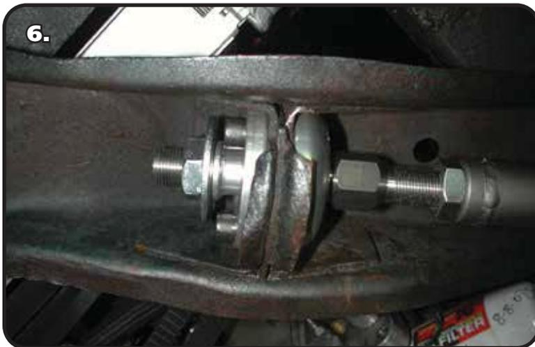
6. Slide the stud through the bearing, then slide the aluminum spacer over the stud with the larger end toward the front of the car. Secure the assembly with a 3/4" Nylok Nut and flat washer. Use **Images 6 & 7** as a guide.
