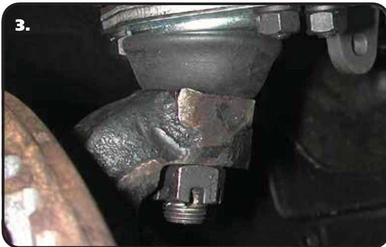
3. Attach the Spindle to the control arms.
