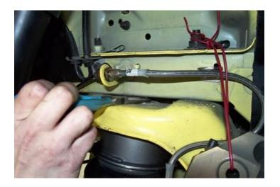
8. Fasten the air spring assembly to the frame in place of the coil spring, using a 7/16" nut and flat washer. The air fitting access should face toward the wheel. It may be easier to use a needle nose pliers to get the nut started on the stud.
