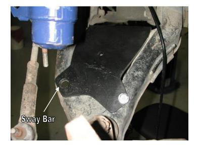
3. Place the lower air spring plate on top of the lower control arm. They are labeled D for driver and P for passenger.
