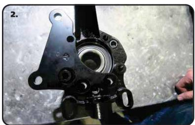
**2.** The caliper brackets are side specific. They have a D & P stamped in them. Lay the correct side caliper bracket on top of the shims, aligning the mounting holes with the mounting holes of the bracket. The counter sunk holes should facing up.
