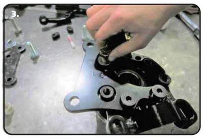
**3.** Insert a 1/2"-13 x 1 1/4" flat head socket cap screw in each of the lower mounting holes. Install a 1/2" flat washer on a 1/2"-13 x 1 1/4" hex bolt and insert it in the upper mounting hole. Tighten the hardware to 75 ft-lbs.
