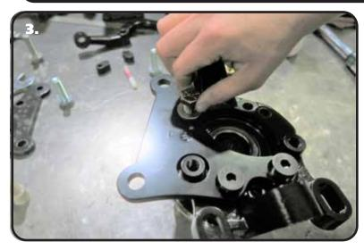
**3.** Insert a  $1/2"-13 \times 1 \ 1/4"$  flat head socket cap screw in each of the lower mounting holes. Install a 1/2" flat washer on a  $1/2"-13 \times 1 \ 1/4"$  hex bolt and insert it in the upper mounting hole. Tighten the hardware to 75 ft-lbs.
