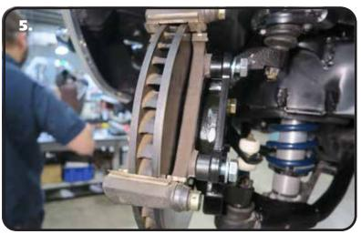
**5.** The OEM caliper bracket will bolt to the spindle mount. Install a M12 flat washer on each of (2) M12-1.75 x 30mm hex bolts. Insert the bolts through the caliper bracket. Line the caliper mount up with the hardware and thread in the bolts.
