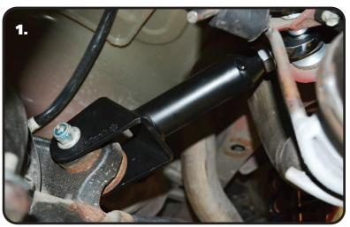
**1.** Install the R-Joint Spacers into the R-Joint End. Remove the OEM Upper Control Arms and replace them with the StrongArms. Tighten the hardware to eliminate any gaps.
