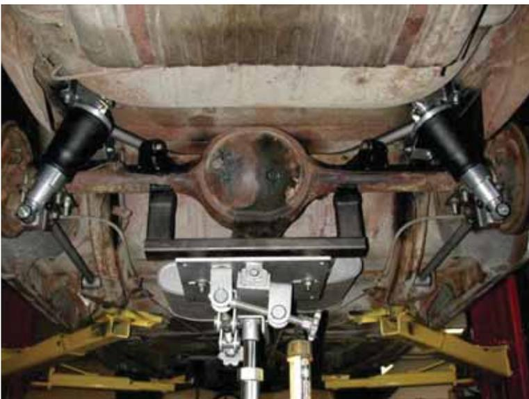
20. Apply thread sealant to the air fitting and screw it into the top of the Shockwave.
