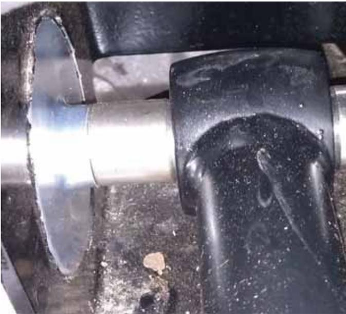
11. With the R-Joint spacers installed, hold the front of the lower bar in the factory leaf spring mount. Install a 9/16" flat washer on each of the (2) 9/16" x 4 1/2" bolts. Insert the 9/16" x 4 1/2" bolt into the LARGE aluminum t-bushing. Insert the bolt/t-bushing through the R-joint/spacers and through the drilled out hole. The Aluminum T-bushing should nest into the leaf spring hole.
