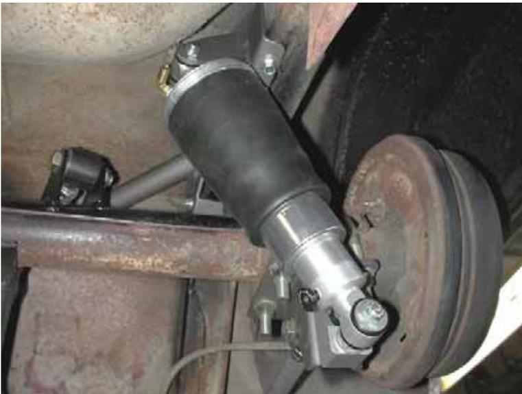
19. This must all be set at **ride height**, which will occur approximately 14.5" from c-c on the shock mounts. As you can see in the above picture, we have tack welded a 5" long spacer between the axle and frame to maintain ride height, axle center, and pinion angle while welding in the tabs.
