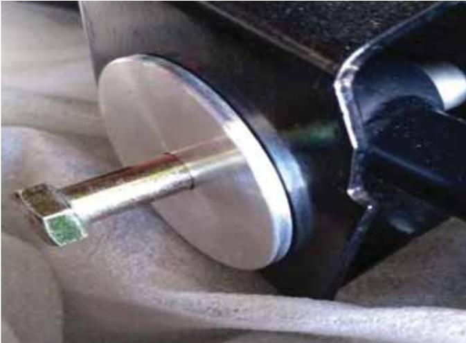
10. The 63-64 years use a 3/4" bolt, it will be replaced with the 9/16" x 4 1/2" bolt supplied in the kit. The bolt hole in the frame will need to be drilled out to 9/16". The Front Lower uses the WIDE(70013768) R-Joint Spacers inserted into each side of the R-Joint with the LARGE Aluminum T-bushing in the leaf spring hole.
