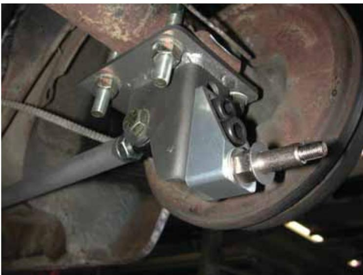
12. Secure the axle mount to the leaf spring pad using the supplied U-bolts. There is an aluminum bushing that will slide over the alignment pin.
