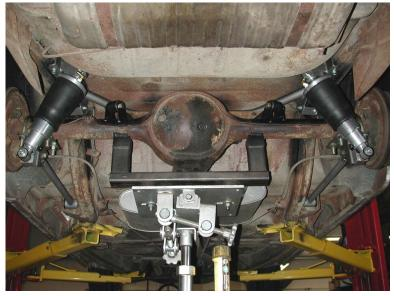
16. Bolt the axle tabs to the upper bar jig using a 5/8" x 2 3/4" bolt and nyloc as shown in the picture. The upper bar should measure 12" C-C.
