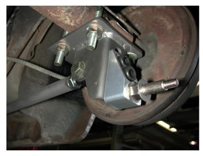
10. The 63-64 years use a 3/4" bolt, it will be replaced with the 9/16" x 4  $\frac{1}{2}$ " bolt supplied in the kit. The bolt hole in the frame will need to be drilled out to 9/16". The Front Lower uses the WIDE(70013768) R-Joint Spacers inserted into each side of the R-Joint with the LARGE Aluminum T-bushing in the leaf spring hole.
