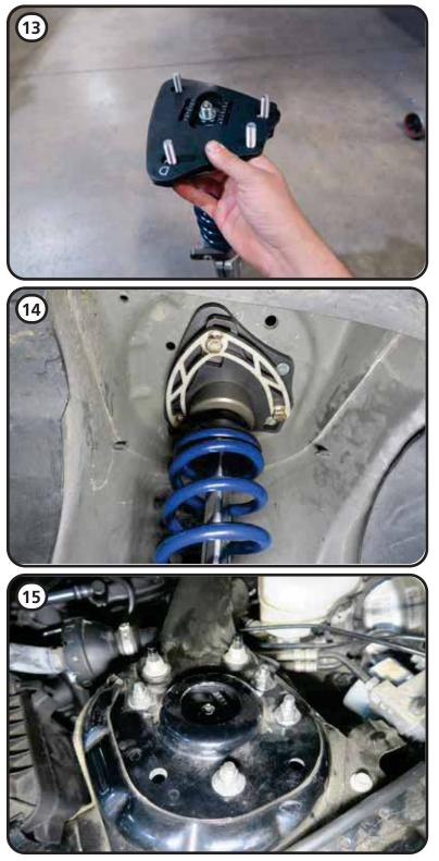
**13.** Image 13 shows the bolt plate inserted with the studs sticking through the bearing plate & caster/camber plate.
