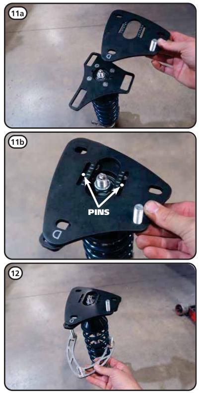
**11a & 11b.** The caster/camber guide plate will sit on top of the bearing plate. The (2) guide pins will get inserted into the slots of the caster/camber guide.
