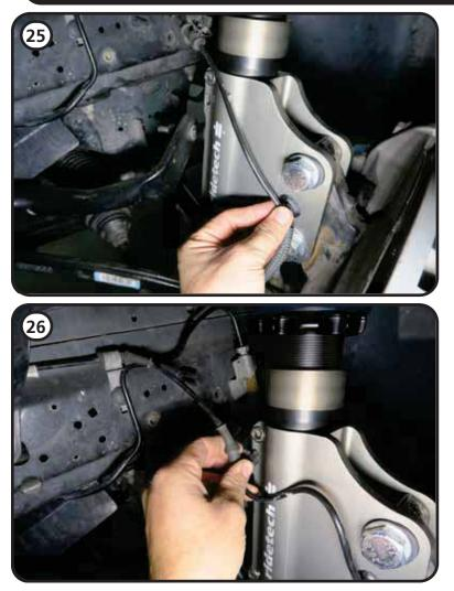
**25.** Attach the outer ABS wire mount to the provision in the tab of the strut.
