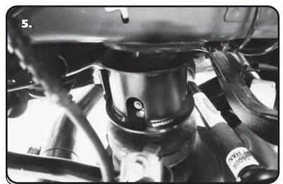
**5.** Install the Air Spring/Upper Cup Assembly into the OEM coil spring location. The top of the Upper Cup will sit in the OEM coil spring location. Clock the fitting to the front of the car, but be sure you have access to it to install the air line. The bottom of the Air Spring will sit on top of the Lower Cup Bracket.
