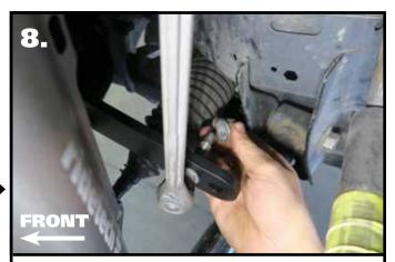
**8.** Install the OEM sway bar linage in the REAR hole of the sway bar. This is a good starting point. See the Sway Bar adjustment note below. Torque the nut to 85 ft-lbs..
