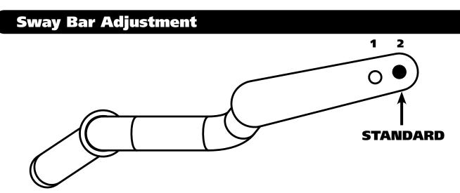
This sway bar has 2 positions to aid in the tuning of your Mustang's handling. We start in the #2 REAR position and tune from there. The #1 position, to the front of the car, will make the sway bar stiffer. The position of the sway bar linkage will be determined by several factors; spring rate, front bar size, and even tire size. Keep in mind, the handling of the car will be affected when you change the linkage location. Drive the car to get accustomed to the new handling characteristics.
