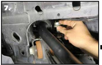
**7.** Reinstall the OEM sway bar mounting hardware. Torque the hardware to 76 ft-lbs.
