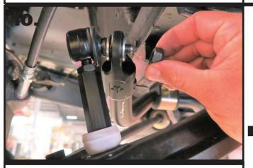
**10.** Insert the 90 degree end link/t-bushing into the swaybar end with the threads pointing toward the engine. Install a 2nd t-bushing with the small diameter into the swaybar. Install the nut and torque. Do this for both sides.
