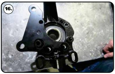
**16.** The caliper brackets are side specific. They have a D & P stamped in them. Lay the correct side caliper bracket on top of the shims, aligning the mounting holes with the mounting holes of the bracket. The counter sunk holes should facing up.
