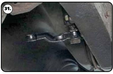
**31.** The TruTurn kit includes a new pitman arm. A pitman arm puller is necessary to replace the pitman arm. Remove the OEM pitman arm using a pitman arm puller. If you do not have one, they can usually be rented from your local auto parts store. Install the new pitman arm using **Image 31** as a reference. The large diameter of the centerlink pin taper should be down toward the ground. Torque the nut 85-110 ftlbs.-+
