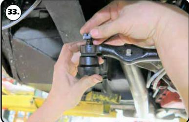
**33.** The other end of the centerlink will sit down on the stud of the idler arm. Install the end of the centerlink on the stud and torque the castle nut to 25-30 ftlbs. Tighten the nut to align the cotter pin. Install the cotter pin and bend the ends.
