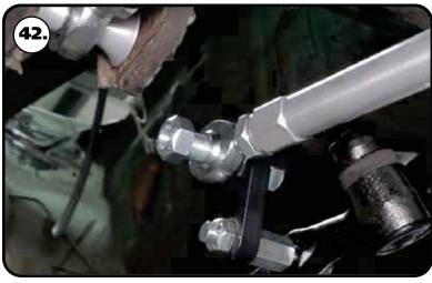
**40.** Install the stud with the round flange into the steering arm with the taper going into the steering arm. Torque the nuts to 35 ftlbs and tighten as needed to align cotter pin hole and install cotter pin.
