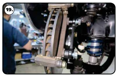
**19.** The OEM caliper bracket will bolt to the spindle mount. Install a M12 flat washer on each of (2) M12-1.75 x 30mm hex bolts. Insert the bolts through the caliper bracket. Line the caliper mount up with the hardware and thread in the bolts.
