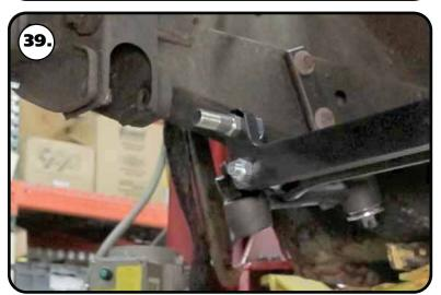
**37.** Install the 1/2"-20 mechanical locking nuts and torque to 50 ftlbs.
