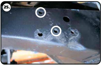
**25.** Remove the idler arm that is currently installed on the car. Your current idler arm may have 3 mounting holes, but there is a 2 hole bolt pattern under it. The idler arm supplied with the kit will use the 2 mounting holes circled in **Image 25**.
