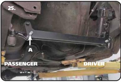
25. The centerlink bracket has one attachment hole [A] that is slotted. This is to accommodate the variations in manufacturing and machining processes, as well as any wear that may have occurred to the original centerlink over time. The slot goes on the passenger side centerlink adapter stud.
