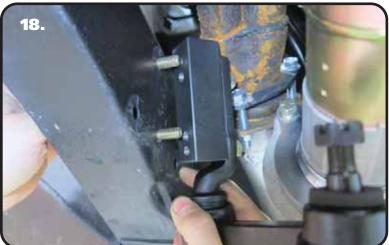
**18.** The idler/spacer is attached to the car using (2) 3/8"-16 x 3 1/4" hex bolts, (2) 3/8" split lock washers, and (2) 3/8" SAE flat washers. Install a 3/8" split lock washer followed by a 3/8" SAE flat washer on each bolt. Insert the bolt/washers into the mounting holes circled in Step 14. Thread the bolts into the 2 top holes of the spacer block. Torque all the 3/8" bolts to 35 ftlbs.
