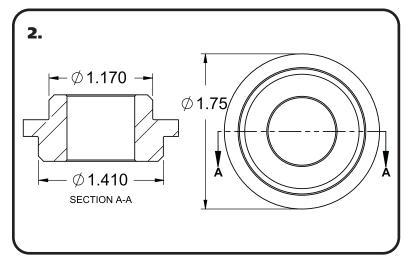
2. This kit includes a t-bushing for the strut rod bushing factory hole. The factory hole can be 2 different diameters depending on the year of the car. The size of your frame hole will determine which direction the t-bushing is installed.
