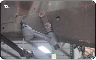
**15.** Attach the new idler arm using the OEM hardware. **Skip to Step 19**.
