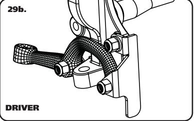
**29a.** Install the steering arms and steering stops onto the spindle using **Images 29a & 29b** as a reference. The steering arms angle toward the centerlink, and the tie rod mounting holes are to the rear of the car. The steering stops are marked D and P.
