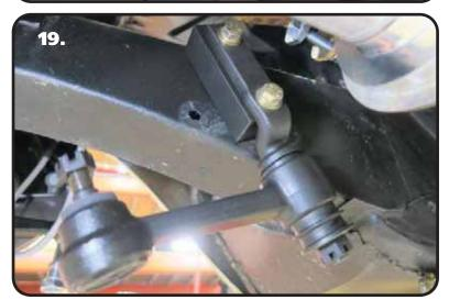
**19.** Install the idler arm on the idler mount with the pin pointing up. Position the pin of the idler to the front of the car before torquing the castle nut. Torque the castle nut to 35-47 ftlbs and tighten to align the cotter pin hole. Install the cotter pin and bend the ends.
