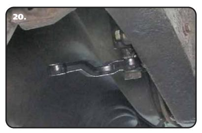
**20.** The TruTurn kit includes a new pitman arm. A pitman arm puller is necessary to replace the pitman arm. Remove the OEM pitman arm using a pitman arm puller. If you do not have one, they can usually be rented from your local auto parts store. Install the new pitman arm using **Image 20** as a reference. The large diameter of the centerlink pin taper should be down toward the ground. Torque the nut 85-110 ftlbs.-+
