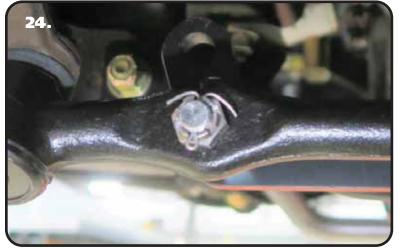
**24.** Torque the nuts to 35 ftlbs and tighten as needed to align cotter pin. Install cotter pin and bend the ends.
