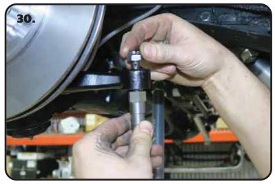
**30.** Install the stud with the round flange into the steering arm with the taper going into the steering arm. Torque the nuts to 35 ftlbs and tighten as needed to align cotter pin hole and install cotter pin.
