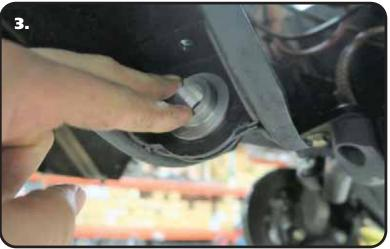
**3.** Test fit the t-bushing in your car's strut rod mount to help determine which direction it needs to be installed. The t-bushing is installed from the front side of the car.
