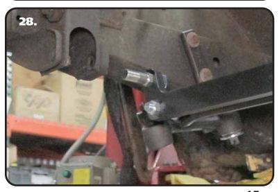
**28.** Install the 5/8"-18 **THIN** mechanical locking nut on the threads of the stud sticking through the centerlink adapter and torque to 45 ftlbs.
