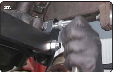
**27.** The studs with the short hex get installed into the centerlink adapter. The short side goes into the adapter attached with the 5/8"-18 thin top lock nut, with the long side of the stud pointing forward.
