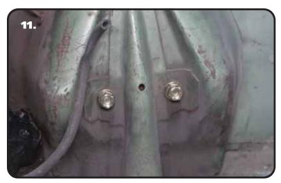
**11.** Install a 1/2" flat washer, 1/2" split lock washer, and 1/2"-13 nut on the threads of the 2 bolts sticking through into the engine compartment. Torque to 75 ftlbs.
