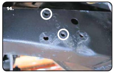
**14.** Remove the idler arm that is currently installed on the car. Your current idler arm may have 3 mounting holes, but there is a 2 hole bolt pattern under it. The idler arm supplied with the kit will use the 2 mounting holes circled in **Image 14**.
