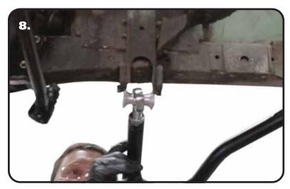
**8.** Install the 2 aluminum spacers into the rod end that goes into the factory control arm pivot. Slip the control arm into the factory frame mount.
