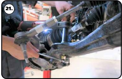
**21.** Install a 1/2" flat washer and 1/2"-13 nylok nut on the threads of each bolt sticking through the control arm. Torque the hardware to 75 ftlbs.
