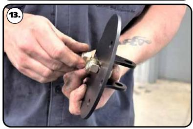
**13.** Install a 1/2" SAE flat washer & 1/2"-13 nylok nut on the threads of each bolt that is sticking through the mount. Torque to 75 ftlbs.
