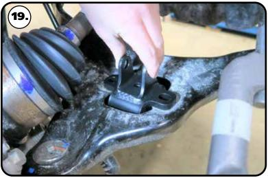
**19.** The lower shock mount bolts to the lower control arm in the same location as the OEM shock. Sit the mount on the lower control arm, aligning the mounting holes with the shock mounting holes
