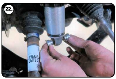
**22.** Install the 1/2" I.D. bearing spacers into bearing in the shock body. These spacers have a through hole that is 1/2" diameter. The small diameter of the spacers will insert into the shock bearing.
