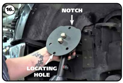
**16.** The upper mount has 4 holes in the perimeter of the flange. The flange is also notched out on one side. The upper mount needs to be installed in the truck with the notch to the frame.
