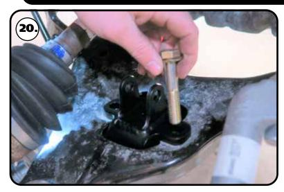
**20.** Install a 1/2" flat washer on each of (2) 1/2"13 x 3" hex bolts. Insert a bolt/washer in each mounting hole.
