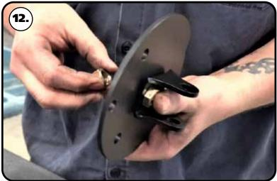
**12.** Insert a 1/2"-13 x 1 1/2" bolt through each hole of the flange/mount. The bolts need to be installed with the bolt head in the upper bracket. Refer to **Images 12 & 13**.
