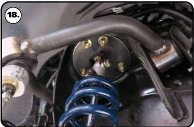
**18.** Install a 7/16" flat washer on each of (4) 7/16"-14 x 1 1/4" hex bolts. Install the bolt/ washer in the frame/mount from the top side with the threads pointing down. Install a 7/16" flat washer and 7/16"-14 nylok nut on the threads of each bolt sticking through the frame. Torque the hardware to 50 ftlbs. Repeat steps 11-18 on the remaining side.
