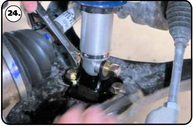
**24.** Install a 1/2" flat washer and 1/2"-13 nylok nut on the threads of the bolt that are sticking through the mount.
