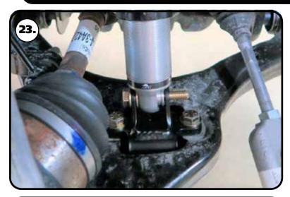
**23.** Insert the shock into the lower mount. Line up the shock bearing/spacers hole with the mounting holes of the lower mount. Insert a 1/2"-13 x 2 3/4" bolt through the mount/ shock.
