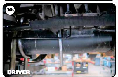
**10.** Install a 7/16" u-bolt on the driver side axle tube just to the outside of the brake line mount.
