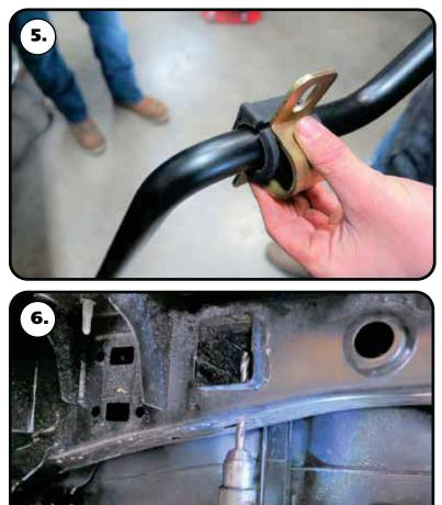
**5.** Install the bushing straps over the sway bar bushings.
