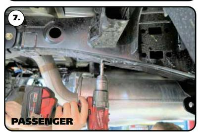
**7.** Drill the passenger side shock crossmember using a 1/2" drill bit. We user the back edge of the frame slot as a guide. Drill the whole straight up from the rear of the frame slot.
