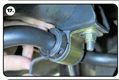
**17.** Install the locking rings on the inside of each bushing assembly. Use a hex key to take the locking ring apart. Reassemble it on the bar positioned next to the inside of the bushing assembly. Push the locking ring up against the bushing assembly and tighten.
