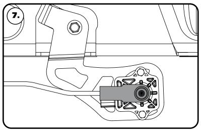
**7.** Reinstall the headlight sensor on the new bracket using the OEM hardware. The new bracket is slotted to allow for adjustment to set the headlights to your new ride height.
