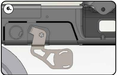
**6.** Install the frame bracket in place of the OEM bracket using the OEM hardware.
