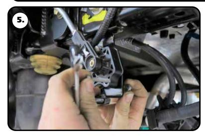
**5.** Remove the headlight sensor from the frame bracket. Unbolt the frame bracket from the fame. Retain the hardware to reinstall the sensor.
