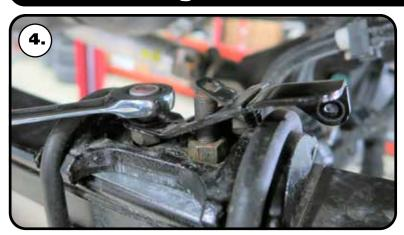
**4.** Disconnect the headlight sensor linkage from the Drivers side leaf spring mount. Remove the linkage bracket from the axle. There isn't a sensor on the Passenger side of the truck.
