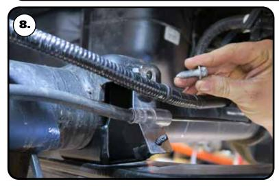
**8.** Remove the brake line bracket bolt from the rear of the drivers side leaf spring pad. Retain the hardware for assembly. If you are using the optional air springs, a longer bolt is supplied.
