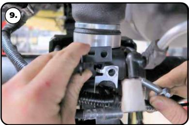
**9.** The lower relocation bracket will get positioned under the brake line mount. The tab of the brake line mount needs to be engaged in the bracket and leaf spring pad. Reinstall the OEM hardware if you're not running the helper air spring kit. If you are using the helper air spring kit, use the supplied M8-1.25 x 30mm bolt and M8 flat washer. Torque to 169 in-lbs.
