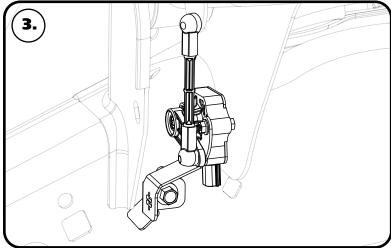
**3.** Reattach the headlight sensor to the new bracket using the OEM hardware.
