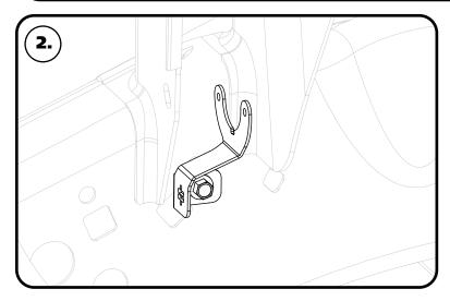
If you are installing the kit on a F150 with headlight sensors, the front headlight sensor bracket will need to be changed. Unbolt the sensor from the front bracket, retaining the hardware. Remove the OEM sensor bracket from the frame and install the need bracket using the OEM hardware.
