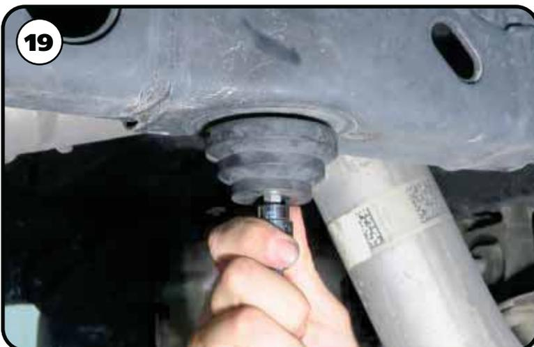
**19.** Install a M10 flat washer on a M10-1.5 x 30 mm socket head cap screw. Insert the washer/bolt in the center hole of the bumpstop. Use a hex key (allen) wrench to attach the bumpstop in the OEM location. Repeat on the other side and torque to 35 in-lbs.
