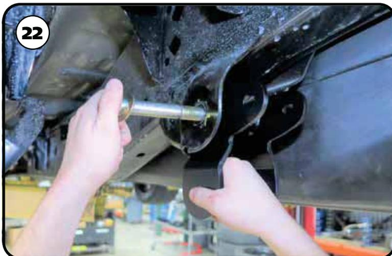
**22.** Install a M18 flat washer on a M18-2.5 x 130mm bolt. Insert the bolt into the OEM leaf spring hole. Install a M18 flat washer & M18-2.5 nylok nut on the threads of the bolt. Do not tighten at this time.
