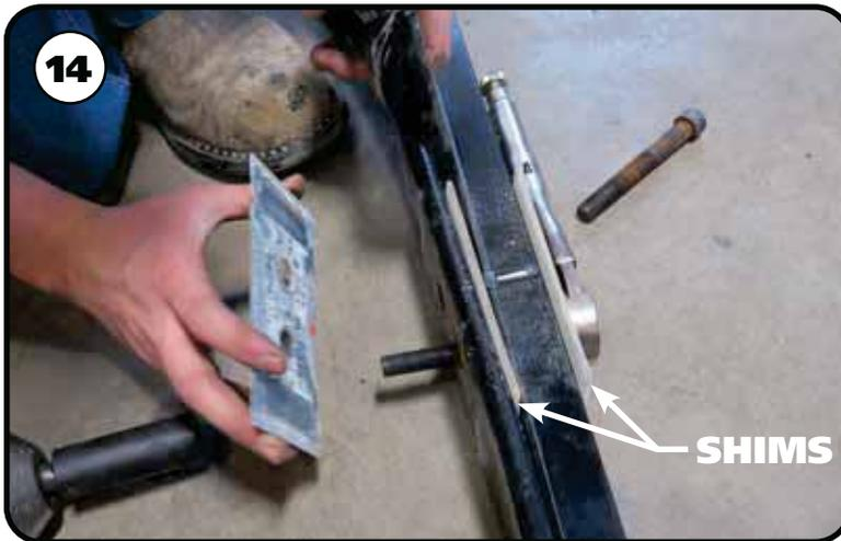
**14.** The top shim will also be discarded. The CENTER & BOTTOM shims will need to be replaced with the offset ones supplied in the kit. **Steps 15 & 16** illustrate the OEM and Offset Shims. Remove the locating pins and remove the shims to prep for flipping the locating pins and replacing the shims.
