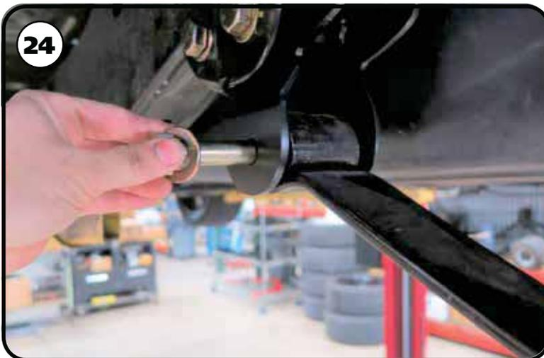
**24.** Insert the front of the leaf spring in the new bracket. Install a M18 flat washer on a M18-2.5 x 130mm bolt. With the mounting holes aligned with the inner sleeve of the leaf spring, insert the bolt/washer. Install a M18 flat washer and M18-2.5 nylok nut on the threads of the bolt. Repeat on the second side. Do not tighten this hardware until the truck is sitting on the ground
