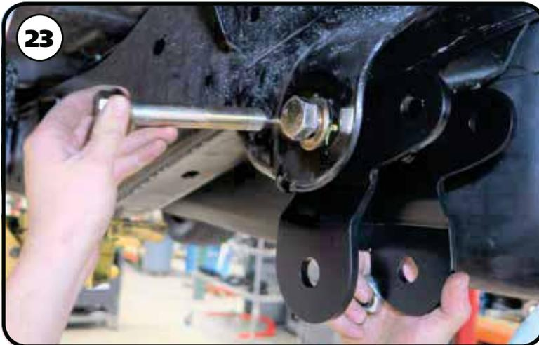
**23.** Make sure the holes in the front tab line up with the front hole of the OEM leaf spring mount. Install a 3/4" flat washer on a 3/4"-16 x 5" bolt. Insert the bolt/washer through the front hole of the leaf spring mount. Install a 3/4" flat washer & 3/4"-16 thin nylok nut on the threads of the bolt. Torque the hardware to 75 ftlbs.
