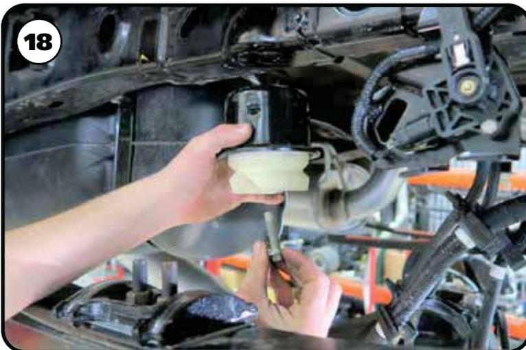
**18.** The OEM bump stop mount will need to be removed.
