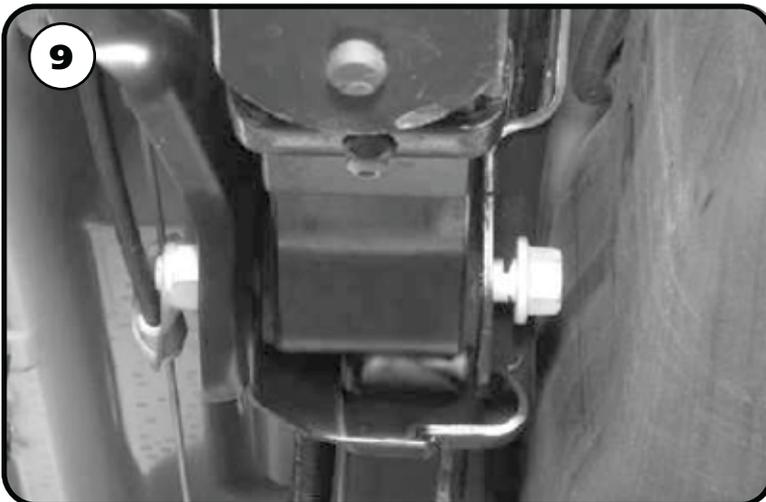
9. The front of the leaf springs will need to be disconnected to install the front bracket and to move the springs under the axle. Due to the location of the fuel tank and exhaust, cutting the bolt head off is the easiest way to remove it. Loosen the nut enough to expose the shank of the bolt. Push the bolt in toward the fuel tank/exhaust. Cut off the head of the bolt, being careful to not damage the fuel tank, exhaust, or frame.
