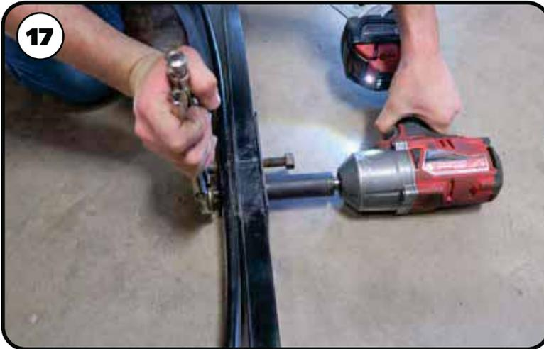
**17.** Put the new offset shims in position with the arrows to the front of the truck. Align the holes in the springs and shims and reinstall the locating pins from the TOP side. Reinstall the nuts on the BOTTOM side and tighten. Torque the nuts to 35 ftlbs. Repeat on the second spring.
