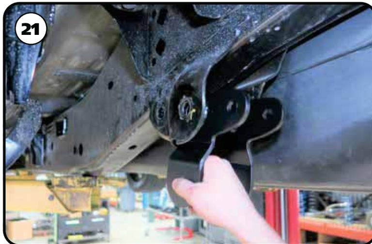
**21.** Insert the leaf spring hanger bracket into the OEM leaf spring mount. The long tabs will point to the front of the truck and insert into the OEM mount. Position the bracket so that the tube lines up with the OEM leaf spring mounting hole.
