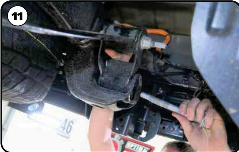
**11.** The rear of the leaf springs will need to be disconnected to move the springs under the axle and to also replace the shackle. Support the rear of the leaf spring and remove the bottom leaf spring shackle bolt. Remove the rear shackle from the leaf spring.
