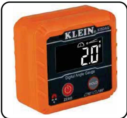
On composite leaf spring trucks, we have found some variation of the pinion angle. When measuring the driveline angles for our flip bracket purposes, we are simply looking at the rear pinion angle. It is important to note that these measurements should be taken at ride height and with the truck on the same surface every time. We used a Klein digital angle finder as shown. **THE PINION ANGLE SHOULD BE APPROXIMATELY 1° DOWN.**
