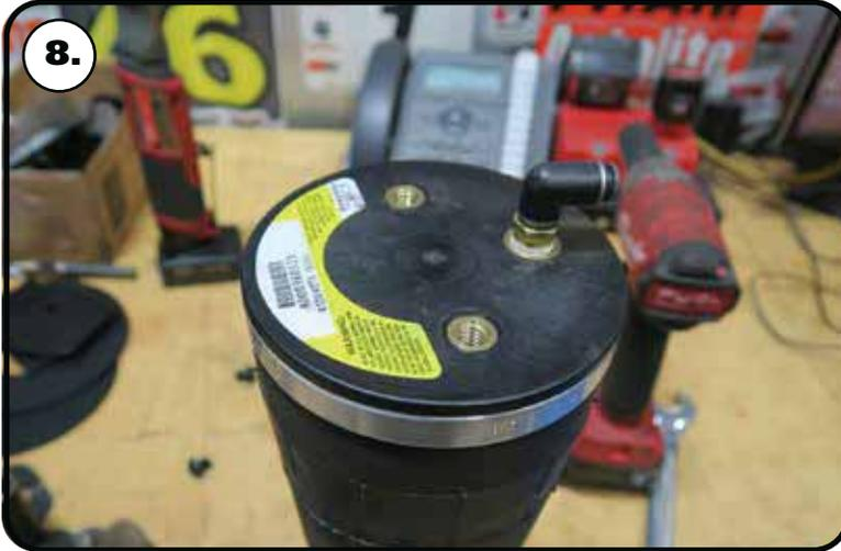
**8.** Put thread sealant on air fittings and thread them into the top of each air spring and tighten.
