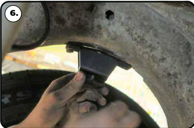
6. Install the bumpstop/mount in the OEM location using the OEM hardware.
