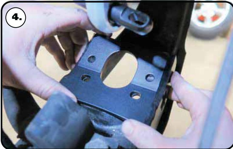
**4.** Lay the lower shock mount on the lower control arm aligning the outer holes with the OEM shock mounting holes. This mount strengthens the control arm and relocates the bottom of the shock toward the engine.
