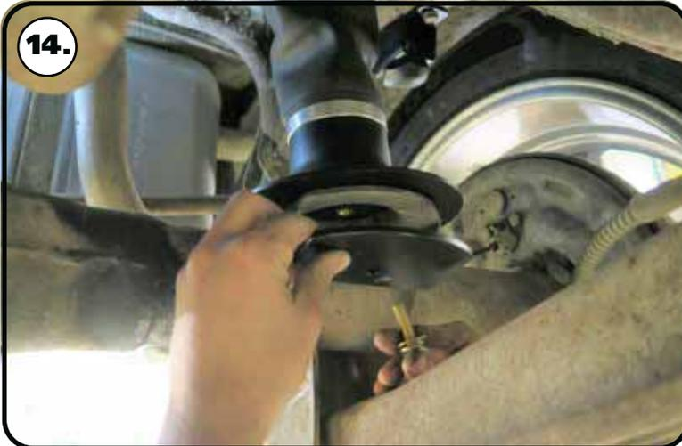
**14.** The "D" shaped clamping plate will clamp the bottom of the air spring in place. The CURVED side of the plate will go to the front of the car, away from the axle tube.
