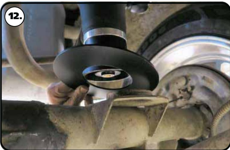
**12.** Install the lower air spring roll plate on the lower coil spring mount. The center hole of the roll plate will sit over the coil spring locator.
