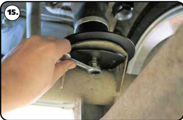
**15.** Install a 3/8" split lock washer & 3/8" SAE flat washer on each a 3/8"-16 x 1" hex bolt. Insert the bolt in the hole of the clamping plate, threading it into the bottom of the air spring. Torque the bolts to 23 ft-lbs.
