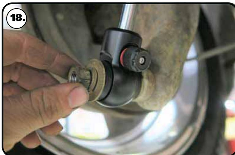
**18.** Attach the eyelet of the shock to the OEM shock stud using the OEM hardware. We recommend positioning the adjuster knob to be inside of the car for easier access. You may need to raise or lower the axle to align the shock eyelet with the shock stud.
