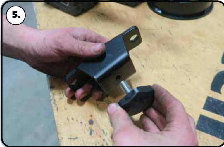
5. Thread the bumpstops in the bumpstop mounts. Thread a 3/8"-16 nut on the threads of the bumpstop. Tighten the nut against the bumpstop mount.
