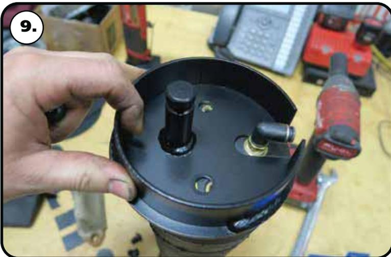
**9.** Align the upper air spring mount with the mounting holes in the top of the air spring. The upper mount is notched out to clear the air fitting. Align the notch with the air fitting and the 2 mounting holes with the mounting holes of the air spring. Install a 3/8" flat washer on each of (2) 3/8"-16 x 1/2" hex bolts. Thread the bolt/washer in the top of the air spring. Torque to 23 ft-lbs.
