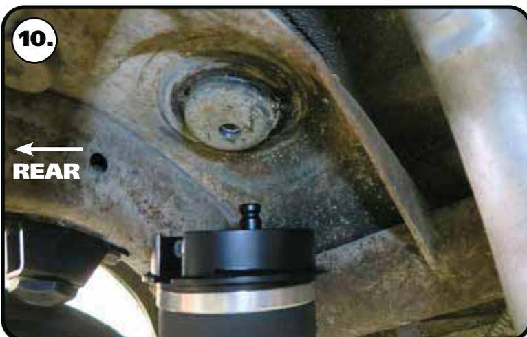
**10.** The pin of the upper air spring will get inserted into the hole drilled in previous steps. The upper mount is positioned in the car with the air fitting to the rear of the car. The pin will go through the center of the spacers installed in **Step 7**.
