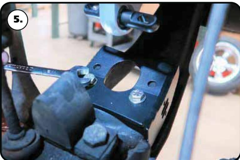
**5.** Install a 5/16" flat washer on each of (2) 5/16"-18 x 1" bolts. Insert the bolt/washer in the aligned holes of the lower mount and control arm. Install a 5/16" flat washer & 5/16" nylok nut on each of the bolts. Torque to 25 ft-lbs.
