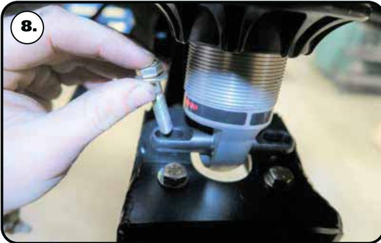
8. Raise the lower arm up to the Shockwave and bolt them together using the 5/16" x 1 1/2" bolts, washers, & nylok nuts supplied with the ShockWaves. Torque to 25 ftlbs.
