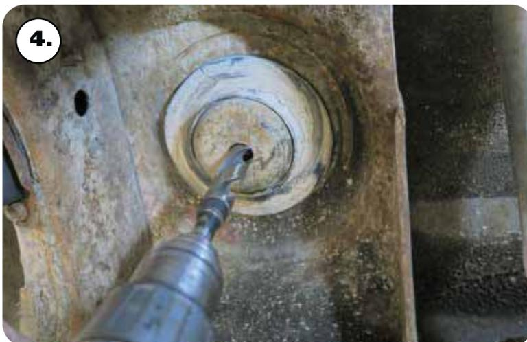
4. Drill a 3/4" hole in the center of the upper coil spring locator. A unibit works well for this.
