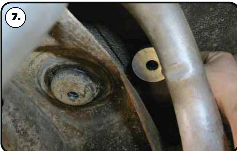
7. Insert the (2) upper mount spacers in the top side of the coil spring locator. The center hole should line up with the hole drilled in **Step 4**.
