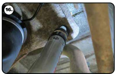
**16.** Use **Images 16 & 17** for proper installation of the shock to the frame of the car. The new shock will be installed in place of the OEM shock. The shock length is designed to work in relation to the air spring stroke length.
