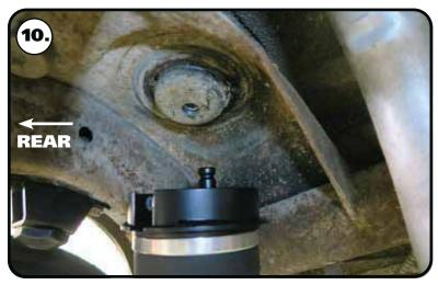
**8.** Put thread sealant on air fittings and thread them into the top of each air spring and tighten.
