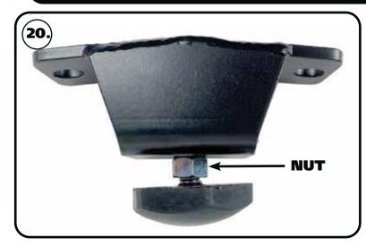
**20.** The bumpstop nut can be moved to the bottom side of the bump stop bracket to limit the amount of compression travel your car has. You can use this to limit how low your car will go when deflated.
