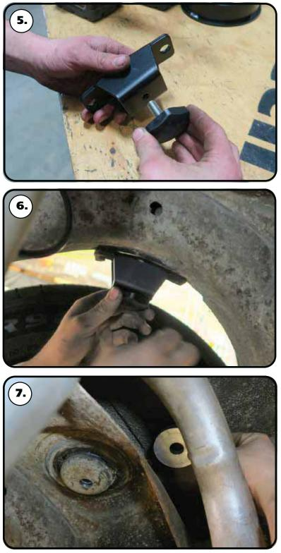
**5.** Thread the bumpstops in the bumpstop mounts. Thread a 3/8"-16 nut on the threads of the bumpstop. Tighten the nut against the bumpstop mount.
