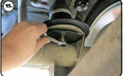
**14.** The "D" shaped clamping plate will clamp the bottom of the air spring in place. The CURVED side of the plate will go to the front of the car, away from the axle tube.
