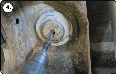
**3.** Remove the bump stops from the OEM location, retaining the OEM hardware. A new bumpstop and bracket will be installed later.
