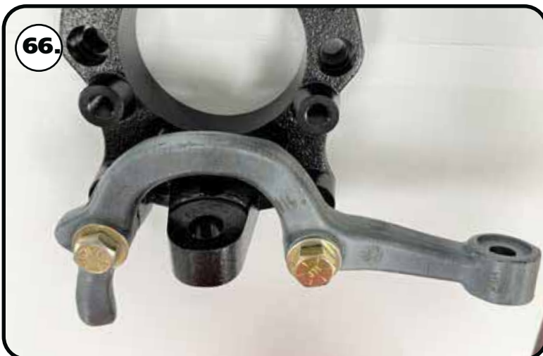
66. Hold the steering arm slugs in place. Align the mounting holes of the steering arm with the threaded holes of the slugs. Driver side steering arm is shown in Image 66 . The tie rod end curves in to the inside of the truck. Install a 1/2" flat washer on a 1/2"-13 x 2" & 1/2"-13 x 2 1/4" hex bolts. The 1/2"-13 x 2 1/4" bolt will go in the hole closest to the tie rod end. Apply red loctite to the threads of the bolts before threading into the slugs. It is the thicker side of the mounts. Insert a bolt in each steering arm hole and thread them into the steering arm slugs. Torque to 80 ft-lbs. Repeat on other steering arm/spindle. Make sure the end of the bolt is sticking out of the slug.
