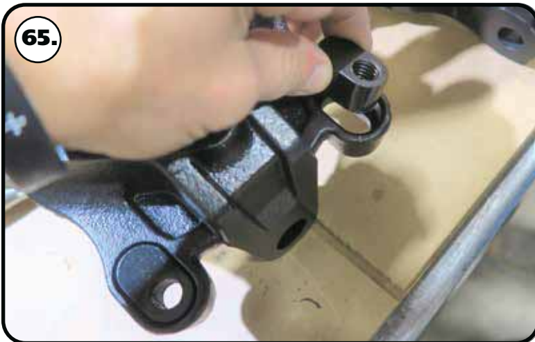
65. Insert the steering arm slugs into the spindle with the threads to the bottom of the spindle,
