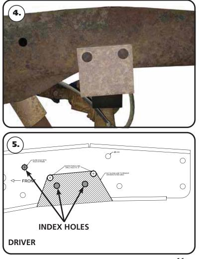
**4.** The OEM bump stop mounts will need to be removed from the frame rail. This can be done by either drilling the rivets out or removing the rivet heads and driving them out. We remove the rivet heads by cutting a "+" in the head with a die grinder then we cut the head off with a hammer and chisel or with an air chisel. Once the head is removed, the rivet can be driven out with a hammer and punch. After removing the frame mounts, drill the rivet holes with a 7/16" drill bit.
