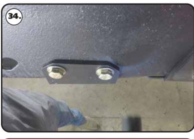
**34.** Install a 7/16" flat washer on each of (4)  $7/16"-14 \times 1/4"$  hex bolts. Insert a bolt/washer in each of the (4) holes. Install a 7/16" flat washer and 7/16"-14 nylok nut on the threads of the bolts. Again, snug the hardware down, but do not torque the hardware at this time. Do this for both sides.
