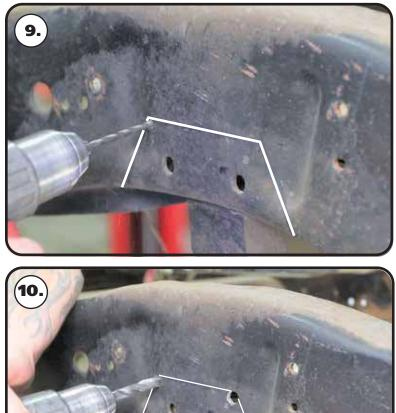
**8.** The corner holes will need to be drill with a 1/2" drill bit, but we recommend drilling the corner holes with a smaller drill bit first.
