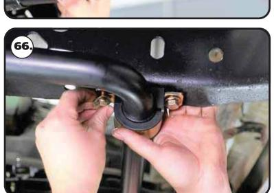
**66.** Install a 3/8" flat washer on each of (4) 3/8"-16 x 1 1/4" hex bolts. Hold the sway bar in place and insert a bolt in the mounting hole of the mounting strap. Install a 3/8" flat washer & 3/8"-16 nylok nut on the threads of the bolt. Repeat this on remaining mounting holes. Do NOT tighten the mounting bolts at this time. They need to left loose until the sway bar linkage has been attached to the lower control arm.
