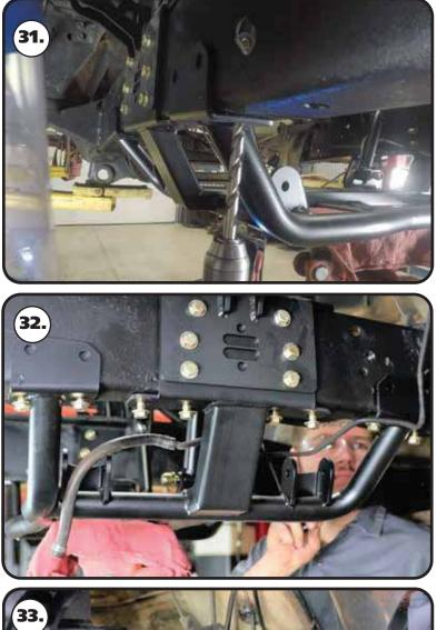
**31.** There are (8) mounting holes in the bottom mounts of each side of the cradle. All but (2) of these will need to be drilled with a 7/16" drill bit. (2) of the holes will align with factory holes.
