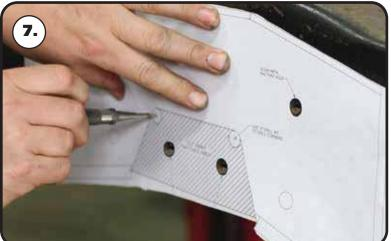
**5.** Cut the indexing holes out of the template and align them with the holes in the frame. We recommend taping the c-notch to the frame to hold it in position.
