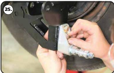
**25.** Insert the bolts through the axle mount and install the flat washers & nylok nuts on the threads sticking through. Repeat on both sides and torque the bolts/nuts to 75 ftlbs. Install a 5/8" flat washer onto the 5/8"-18 threads of the shock stud. Apply Red Loctite to the 5/8" threads of the stud. Thread the shock stud into the threaded hole of the lower mount. Repeat on both sides and torque the shock stud to 65-75 ftlbs.
