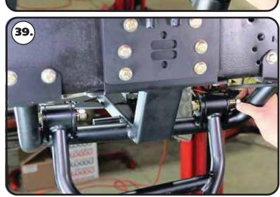
**39.** Install a 1/2" flat washer on each of (2) 1/2"-13 x 3 1/2" hex bolts. Insert the bolt/washer in the aligned holes with the threads to the rear of the truck. Install a 1/2" flat washer & 1/2"-13 nylok nut on the threads of the bolts. Re peat on the passenger side control arm. Torque the mounting bolts to 75 ft-lbs.
