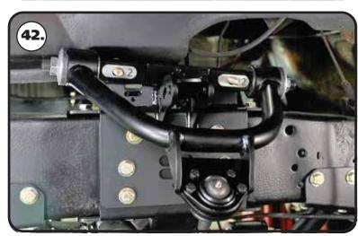
**42.** Insert the caster slug into the cross shaft using the guide on *Page 21* as a guide. *The long side of the caster slug will be to the rear of the control arm.* Slip the upper control arm onto the mounting bolts using *Page 22* as a guide for cross shaft orientation. Install a 7/16" flat washer & 7/16"-14 on the threads of each bolt. Torque the bolts to 70 ft-lbs.
