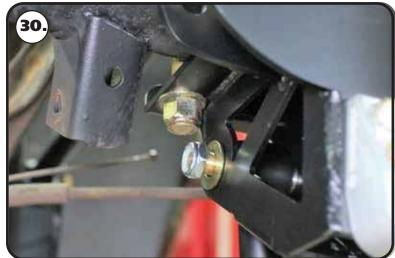
**30.** Line the through hole of the R-Joint with the of holes of the bar mount. Install a 5/8" flat washer on to a 5/8"-18 x 3 1/4" Hex bolt, insert into the lined up holes. Install a 5/8" flat washer followed by a 5/8"-18 THIN nylok nut. Repeat on both sides and tighten the bolts/nuts enough to eliminate any gaps.
