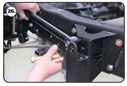
**26.** Insert (2) .625" ID x .740" long R-Joint spacers into the R-Joint of one end of each 23 7/8" center to center upper bar. The small diameter of the spacer goes into the R-joint. Insert the front of the upper bar R-Joint into the front mount. The front mount has 2 bar mounting locations. The 23 3/8" upper bar needs to be installed into the top position.
