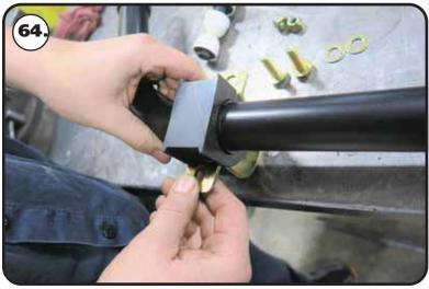
**64.** Install the bushing mounting strap on the sway bar bushing.
