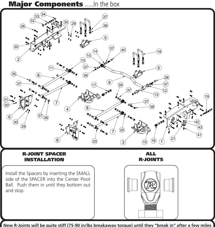
New R-Joints will be quite stiff (75-90 in/lbs breakaway torque) until they "break in" after a few miles of use. After the break in period they will move much more freely. Because the composite bearing race contains self lubricating ingredients, no additional lubrication is needed or desired. Any additional lubrication will only serve to attract more dirt and debris to the R-Joint and actually shorten its life.
