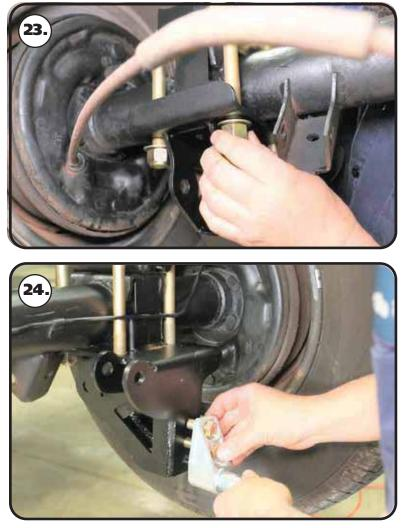
**23.** Hold the mount in place and install a 5/8" flat washer and 5/8"-18 nylok nut on the threads of the u-bolts sticking through the axle mount. Tighten the nuts evenly in a criss-cross fashion making sure the tabs of the axle mount are touching the leaf spring pad evenly. Torque the nuts in a criss-cross fashion to 75 ftlbs. Repeat on the other side.
