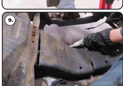
**9.** The OEM i-beam cross member will need to be cut out of the truck. It needs to be cut out even with the top of the frame rail. We also cut the cross member in the center for easier removal. We used a saw-z-all to cut the cross member out of the truck.
