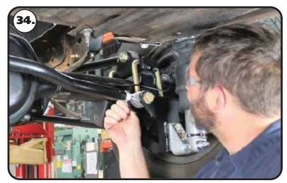
**34.** We used a die-grinder with a cutoff wheel to cut the brake line bracket off the axle tube. Be careful to not cut into the axle tube.
