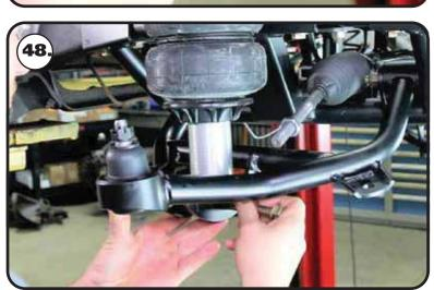
**48.** Install a 1/2" flat washer on a 1/2"-13 x 3" hex bolt. Insert the bolt/washer into the mount/shock. Install a 1/2" flat washer & 1/2"-13 nylok nut. Torque the hardware to 75 ft-lbs.
