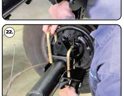
**22.** Install a supplied 5/8" u-bolt in each side of the upper bar mount. The u-bolts will nest in the slots of the upper mount. The U-bolts will run parallel to the axle tube.
