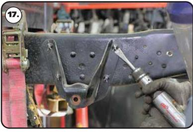
**17.** The OEM front leaf spring mounts will need to be removed from the frame rail. This can be done by either drilling the rivets out or removing the rivet heads and driving them out. We remove the rivet heads by cutting a "+" in the head with a die grinder then we cut the head off with a hammer and chisel or with an air chisel.
