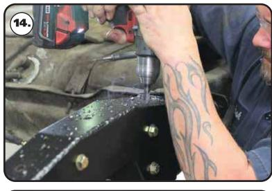
**14.** Use a 7/16" drill bit to drill the remaining holes in the top and bottom of the frame.
