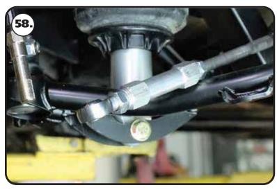
**58.** The tie rod adjusters have (2) different thread sizes, 5/8"-18 LH & 9/16"-18. The left hand threaded heim will thread into the 5/8"-18 end. The rack threads into the 9/16"-18 end. Install the 5/8"-18 LH jam nut on the heim end. Install a 9/16"-18 jam nut on the threads of the rack. Thread the heim into the adjuster and thread the adjuster onto the rack.
