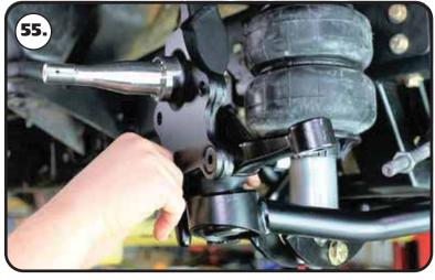
**55.** Install The steering arms on the spindles. The steering arms bolt to the bottom 2 holes of the spindle. The steering arms angle toward the rack, and the tie rod mounting holes are to the front of the truck. The steering arm attaching hardware is supplied with the spindle.
