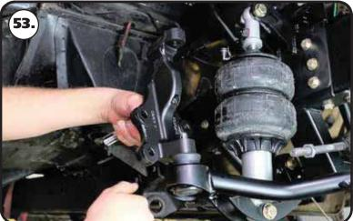
**53. THESE SPINDLES ARE SYMMETRICAL, THEY AREN'T SIDE SPECIFIC UNTIL THE STEERING ARM IS BOLTED ON.** Install the spindle on the lower ball joint. Install the ball joint castle nut on the stud of the ball joint.
