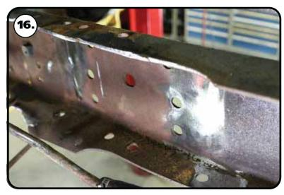
**16.** The inside of the frame rails need to be ground smooth.
