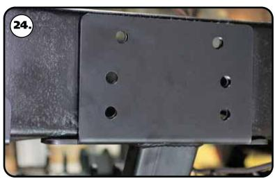
**24.** Position the cradle so that the (6) holes of the side plate align with the rivet holes in the frame.
