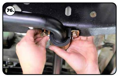
**76.** Install a 3/8" flat washer on each of (4) 3/8"-16 x 1 1/4" hex bolts. Hold the sway bar in place and insert a bolt in the mounting hole of the mounting strap. Install a 3/8" flat washer & 3/8"-16 nylok nut on the threads of the bolt. Repeat this on remaining mounting holes. Do NOT tighten the mounting bolts at this time. They need to left loose until the sway bar linkage has been attached to the lower control arm.
