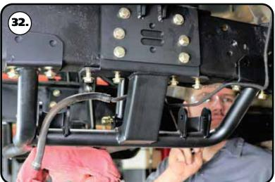
**32.** Install a 7/16" flat washer on each of (8) 7/16"- $14 \times 1$  /4" hex bolts. Insert a bolt/washer in each bottom (8) holes. Install a 7/16" flat washer and 7/16"-14 nylok nut on the threads of the bolts. Again, snug the hardware down, but do not torque the hardware at this time. Do this for both sides.
