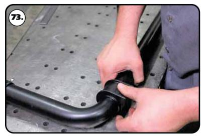
**73.** Open the sway bar bushing at the split and slip it onto the sway bar. Do this for both bushings.
