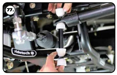
**77.** Install the end links using **Diagram 67** as a reference. Install both end links before tightening the end link hardware.
