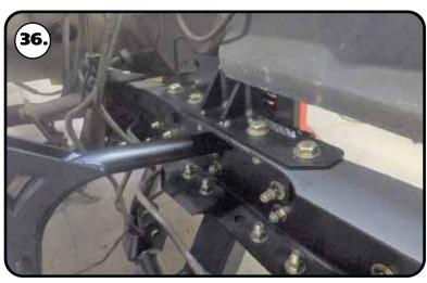
**36.** Install a 7/16" flat washer on each of (4) 7/16"-14 x 1 /4" hex bolts. Insert a bolt/washer in each top (4) holes. Install a 7/16" flat washer and 7/16"-14 nylok nut on the threads of the bolts. Torque all 7/16" cradle hardware to 70 ft-lbs. Torque the 1/2" engine mount hardware to 75 ft-lbs.
