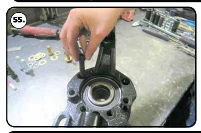
**55.** The Hub is attached to the spindle using  $(4) M12-1.50 \times 40 SHCS$ . Apply RED Loctite to each of the mounting bolts. Insert them into the correct holes and Torque to 99 ftlbs.
