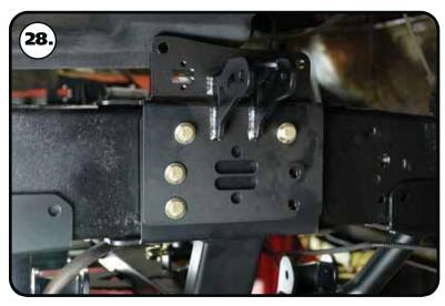
**28.** Install a 7/16" flat washer on a 7/16"-14 x 1 3/4" hex bolt. Insert the bolt in the top hole of the rear (3) bolt holes. This bolt will go through the upper control arm mount, cradle plate, & engine mount. Install a 7/16" flat washer and 7/16"-14 nylok nut on the threads of the bolt. DO NOT INSTALL A BOLT IN THE LOWER HOLE OF THE ENGINE MOUNT HOLE AT THIS TIME.
