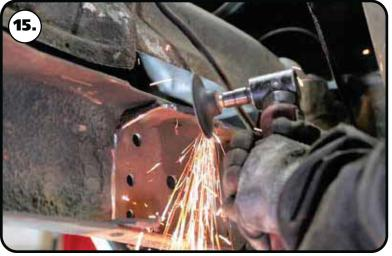
**15.** We grind the top of the cross member back to the frame rail.
