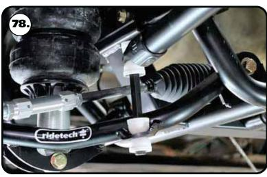
**78.** Tighten the end link barrel nut until it is flush with the end of the bolt, and then tighten it 2-3 more complete rounds. Torque the frame bolts to 45 ft-lbs.
