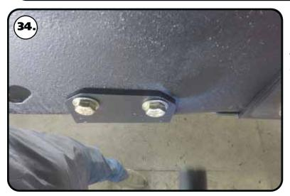
**34.** Install a 7/16" flat washer on each of (4) 7/16"- $14 \times 1$  /4" hex bolts. Insert a bolt/washer in each of the (4) holes. Install a 7/16" flat washer and 7/16"-14 nylok nut on the threads of the bolts. Again, snug the hardware down, but do not torque the hardware at this time. Do this for both sides.
