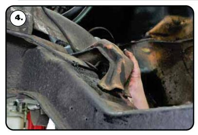
**4.** Remove the OEM engine mount stands.
