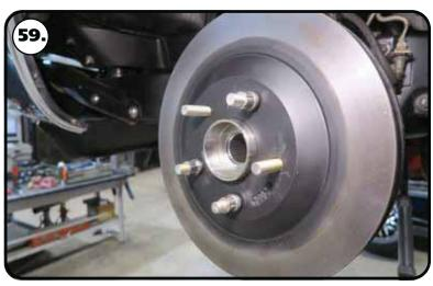
**59.** Install the rotor on the hub. Thread some lug nuts on the threads of the hub to hold the rotor tight on the hub.
