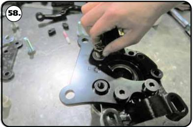
**58.** Insert a  $1/2"-13 \times 1 \ 1/4"$  flat head socket cap screw in each of the lower mounting holes. Install a 1/2" flat washer on a  $1/2"-13 \times 1 \ 1/4"$  hex bolt and insert it in the upper mounting hole. Tighten the hardware to 75 ft-lbs.
