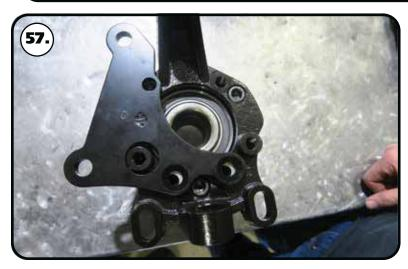
**57** The caliper brackets are side specific. They have a D & P stamped in them. Lay the correct side caliper bracket on top of the shims, aligning the mounting holes with the mounting holes of the bracket. The counter sunk holes should facing up.
