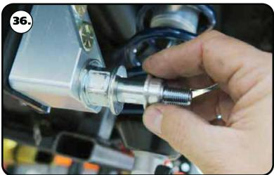
are .400" long (90002067). Install a 5/8" ID 90002067 spacer (Small side towards shock body) onto the lower Shock Stud. Slide the bottom of the Shock onto the Stud. Install a second 5/8" ID 90002067 Spacer onto the Stud (small side towards shock). You may need to jack the rear end up to Slide the Shock onto the Stud.
