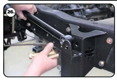
**26.** Insert (2) .625" ID x .740" long R-Joint spacers into the R-Joint of one end of each 23 7/8" center to center upper bar. The small diameter of the spacer goes into the R-joint. Insert the front of the upper bar R-Joint into the front mount. The front mount has 2 bar mounting locations. The 23 7/8" upper bar needs to be installed into the top position.
