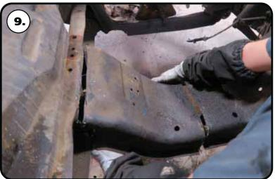
**9.** The OEM i-beam cross member will need to be cut out of the truck. It needs to be cut out even with the top of the frame rail. We also cut the cross member in the center for easier removal. We used a saw-z-all to cut the cross member out of the truck.
