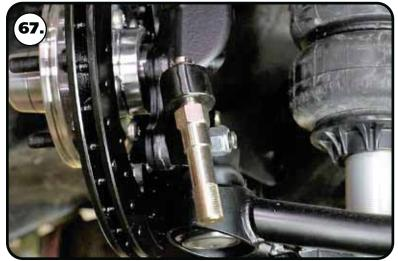
**67.** Install the stud with the hex into the steering arm with the taper going into the steering arm. Install the 7/16"-20 castle nut onto the tie rod stud. Torque the nuts to 35 ftlbs and tighten as needed to align cotter pin hole and install cotter pin.
