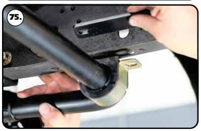
**75.** The sway bar includes a backer plate that needs to be installed on the top side of the frame flange. Align the backer plate holes with the holes drilled in the frame.
