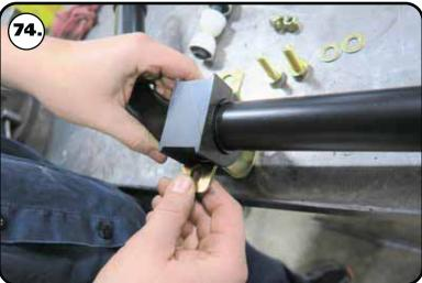
**74.** Install the bushing mounting strap on the sway bar bushing.
