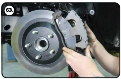
**62.** Install the brake pads and caliper.
