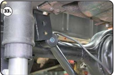
**33.** Remove the bolt that attaches the brake hose to the bracket. This will allow you to move the brake line out of the way to cut the bracket off the axle tube.
