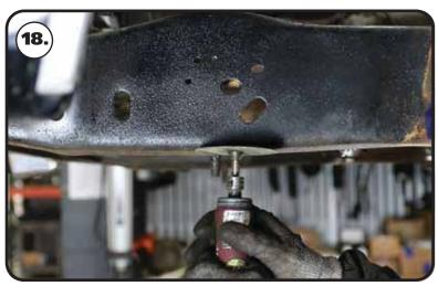
**18.** There is a pin that sticks down from the bottom of each frame rail that needs to be removed. These pins are in front of the OEM cross member. These need to be cut off even with the frame rail.
