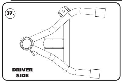
**37.** The lower control arms are marked "D" for Driver and "P" for Passenger. The ball joint pin points up and the sway bar mount is on the front side of the arm. **Diagram 37** shows a top view of the Driver lower control arm.
