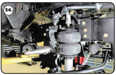
**54.** Insert the top ball joint into the spindle.
