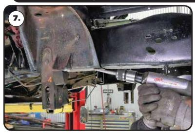
**7.** Remove the side and bottom rivets from the frame mounts.
