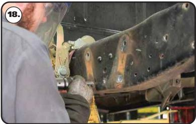
**18.** Once the head is removed, the rivet can be driven out with a hammer and punch. After removing the frame mounts, drill the rivet holes with a 7/16" drill bit.
