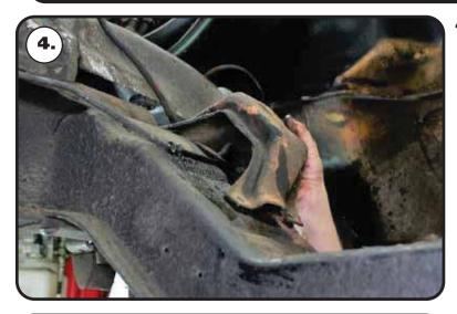
**4.** Remove the OEM engine mount stands.
