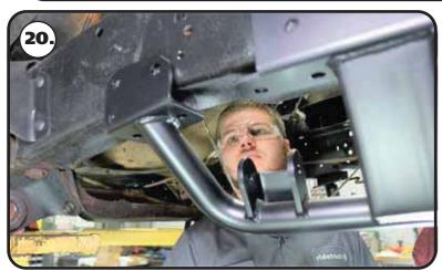
**20.** The 73-79 F100 trucks passenger frame rail has a section of the frame bent downward. This bent down area is in the location of the rear crossmember mount. This area needs to be flattened for cradle installation. The cradle can be lifted in position to mark the area that needs flattened
