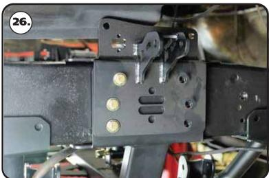
**26.** Install a 7/16" flat washer on each of (3) 7/16"-14 x 1 /4" hex bolts. Insert a bolt in the front (3) bolt holes. Install a 7/16" flat washer and 7/16"-14 nylok nut on the threads of the bolt. This will help keep everything aligned. Do this for both sides.
