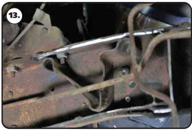
**13.** Remove the steering box inner spacer. This mount can be removed by straightening the (2) tabs that stick through the frame.
