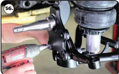
**56.** Insert the 1/2"-20 flat head bolts in front the wheel side of the spindle. The 1/2"-20 nylok nuts will go against the steering arm. Torque the hardware the 100 ftlbs.
