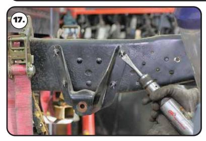
17. The OEM front leaf spring mounts will need to be removed from the frame rail. This can be done by either drilling the rivets out or removing the rivet heads and driving them out. We remove the rivet heads by cutting a "+" in the head with a die grinder then we cut the head off with a hammer and chisel or with an air chisel.
