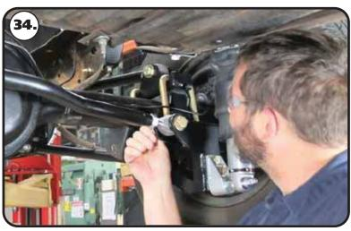
**34.** We used a die-grinder with a cutoff wheel to cut the brake line bracket off the axle tube. Be careful to not cut into the axle tube.
