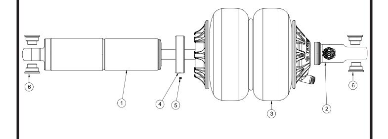
WARNING: ATTEMPTING TO REMOVE THE AIR FITTING WILL DAMAGE IT AND VOID THE WARRANTY.
