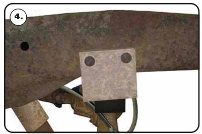
**4.** The OEM bump stop mounts will need to be removed from the frame rail. This can be done by either drilling the rivets out or removing the rivet heads and driving them out. We remove the rivet heads by cutting a " + " in the head with a die grinder then we cut the head off with a hammer and chisel or with an air chisel. Once the head is removed, the rivet can be driven out with a hammer and punch. After removing the frame mounts, drill the rivet holes with a 7/16" drill bit.
