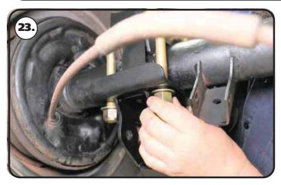
23. Hold the mount in place and install a 5/8" flat washer and 5/8"-18 nylok nut on the threads of the u-bolts sticking through the axle mount. Tighten the nuts evenly in a criss-cross fashion making sure the tabs of the axle mount are touching the leaf spring pad evenly. Torque the nuts in a criss-cross fashion to 75 ftlbs. Repeat on the other side.
