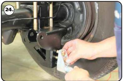
**24.** The lower shock mount attaches with (1) 1/2"-13 x 1 1/4" hex bolt, (1) 1/3"-13 x 1 3/4" hex bolt, & (2) 1/2" flat washer, & (2) 1/2"-13 nylok nuts. The lower mount gets attached to the 2nd and 3rd hole up from the bottom of the axle mount. When the shock mount is installed correctly, the bottom of the lower shock mount is 1/2" below the bottom of the axle mount. Insert the bolts through the aluminum shock mount with the 1 1/4" long bolt in the top hole, 1 3/4" in the bottom hole.
