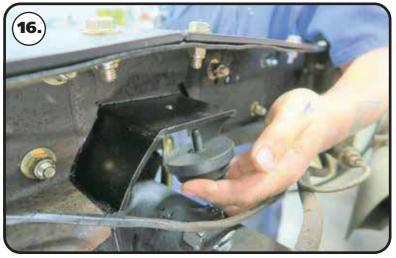
**16.** Install the bump stop using a 3/8"-16 x 1" socket head bolt, 3/8" flat washer, & 3/8"-16 nylok nut. Hold the bump stop with your hand and insert the bolt through the center of the bump stop. Line up the bolt of the bump with the drilled hole of the frame. Install a 3/8" flat washer and 3/8" nut on the threads of the bolt. Tighten to 60 **in-lbs**.
