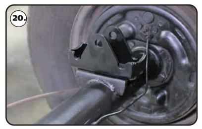
**20.** Sit the upper bar mount on the leaf spring pad of the axle. The locating pin needs to insert into the leaf spring locating hole of the leaf spring pad.
