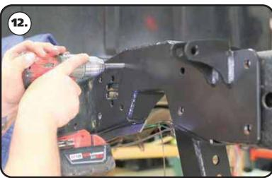
**12.** After cutting, slip the c-notch over the frame to check the fitment. The cut areas of the frame may require grinding for the c-notch to fit. The c-notch will be used as a template to drill the remaining mounting holes. Use a 7/16" Drill bit to drill the holes in the side of the frame. There are 8 holes in the side that need to be drilled.
