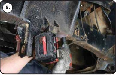
**5.** The bottom rear of the OEM crossmember may have a bolt instead of a rivet. If so, remove the bolt.
