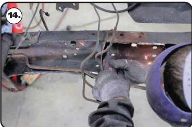
**14.** The vertical sections that are inside the frame rail need to be removed. The frame surface needs to be flat. We cut these out using a die grinder and cut off wheel.
