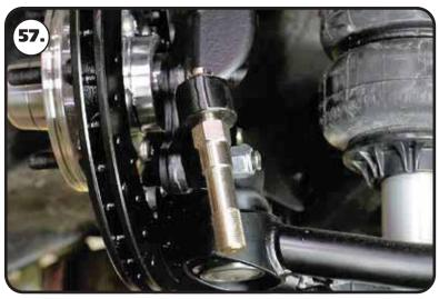
**57.** Install the stud with the hex into the steering arm with the taper going into the steering arm. Install the 7/16"-20 castle nut onto the tie rod stud. Torque the nuts to 35 ftlbs and tighten as needed to align cotter pin hole and install cotter pin.
