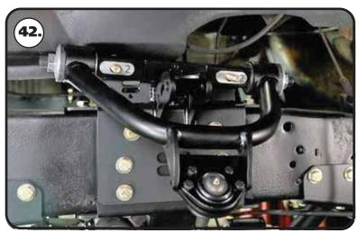
**42.** Insert the caster slug into the cross shaft using the guide on *Page 21* as a guide. *The long side of the caster slug will be to the rear of the control arm.* Slip the upper control arm onto the mounting bolts using *Page 22* as a guide for cross shaft orientation. Install a 7/16" flat washer & 7/16"-14 on the threads of each bolt. Torque the bolts to 70 ft-lbs.
