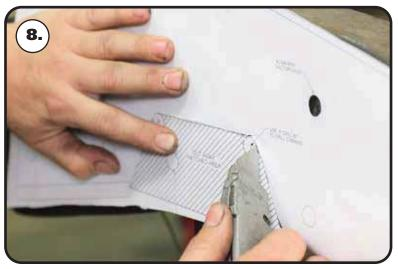
**7.** Use a razor knife to cut along the outer lines of the hashed area of the template. With the hashed area cut out, use the template to mark the frame rail for cutting the c-notch.
