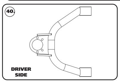
**40.** The upper control arms are marked "D" for Driver and "P" for Passenger. The ball joint pin points down and the ball joint is to the rear of the truck. **Diagram 40** shows a top view of the Driver upper control arm.
