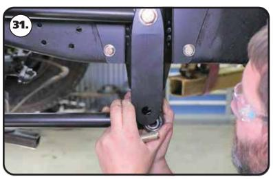
**31.** Insert (2) .625" ID x .740" long R-Joint spacers into the front R-Joint of each lower bar. The small diameter of the spacer goes into the R-joint. Insert the front lower bar R-Joint into the lower position of the frame mount.
