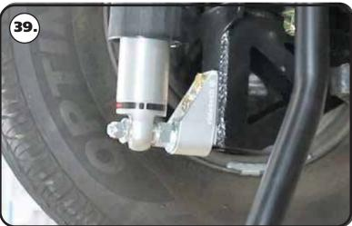
**39.** Install the 7/16" Flat washer and 7/16" Nylok nut. Tighten the upper and lower shock bolts. Torque the Upper Bolt to 50 ftlbs and the Lower Nut to 40 ftlbs. The designed ride height of the CoilOver/Shockwave is 14 1/2" center to center.
