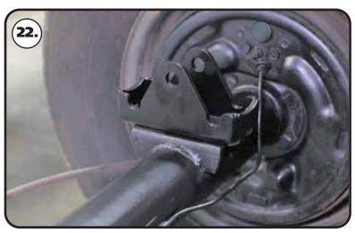
**22.** Sit the upper bar mount on the leaf spring pad of the axle. The locating pin needs to insert into the leaf spring locating hole of the leaf spring pad.
