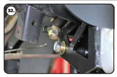
**32.** Line the through hole of the R-Joint with the of holes of the bar mount. Install a 5/8" flat washer on to a 5/8"-18 x 3 1/4" Hex bolt, insert into the lined up holes. Install a 5/8" flat washer followed by a 5/8"-18 THIN nylok nut. Repeat on both sides and tighten the bolts/nuts enough to eliminate any gaps.
