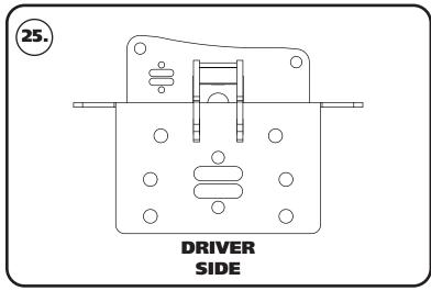
**25.** *Diagram 25* illustrates the Driver side upper control arm mount. This mount is mounted on the outside of the frame, over top the cradle The (6) holes of the upper control arm mount, align with the cradle and frame holes.
