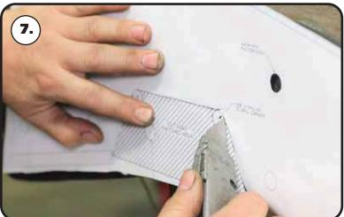
**7.** Use a razor knife to cut along the outer lines of the hashed area of the template. With the hashed area cut out, use the template to mark the frame rail for cutting the c-notch.
