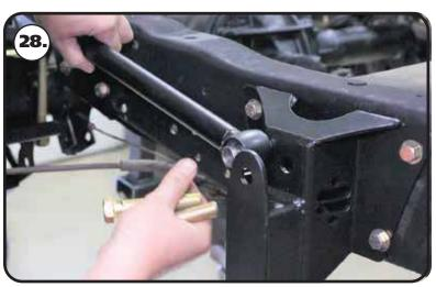
**28.** Insert (2) .625" ID x .740" long R-Joint spacers into the R-Joint of one end of each 23 3/8" center to center upper bar. The small diameter of the spacer goes into the R-joint. Insert the front of the upper bar R-Joint into the front mount. The front mount has 2 bar mounting locations. The 23 3/8" upper bar needs to be installed into the top position.
