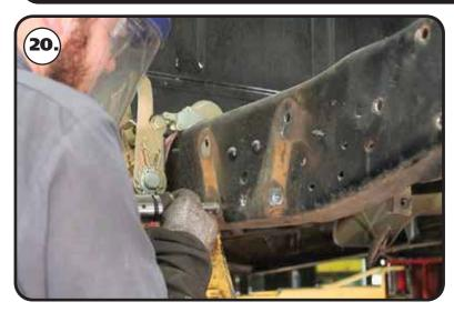
**20.** Once the head is removed, the rivet can be driven out with a hammer and punch. After removing the frame mounts, drill the rivet holes with a 7/16" drill bit.
