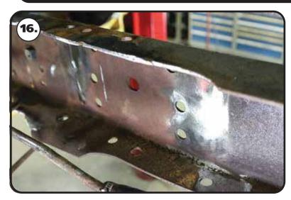
**16.** The inside of the frame rails need to be ground smooth.
