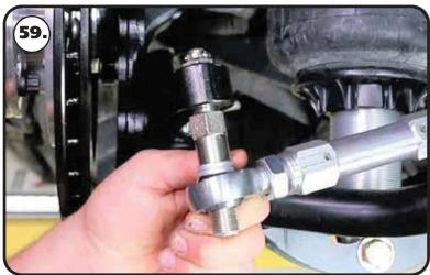
**59.** Install (2) 1/8" thick aluminum spacers on the tie rod stud. Next, slip the heim end onto the tie rod stud.
