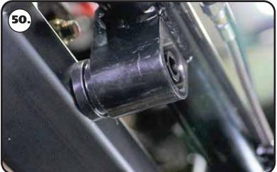
**50.** Install the rack on the bushing half. The steering shaft will be on the drivers side with the shaft pointing toward the cab.
