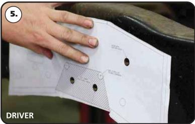
**5.** Cut the indexing holes out of the template and align them with the holes in the frame. We recommend taping the c-notch to the frame to hold it in position.
