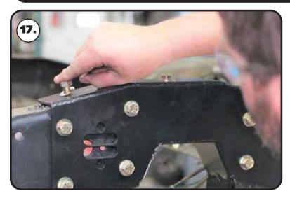
**17.** Install a 7/16" flat washer on each of (5) 7/16" x 1 1/4" bolts. This hardware gets installed in the top & bottom of the c-notch. Install a 7/16" flat washer and 7/16" nylok nut on each bolt sticking through the frame. Tighten the c-notch mounting hardware to 70 ft-lbs.
