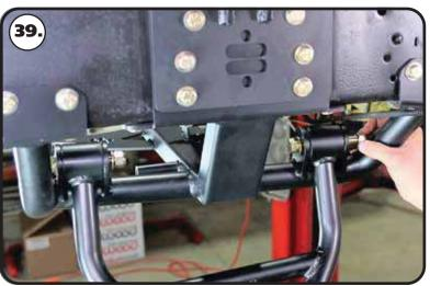
**39.** Install a 1/2" flat washer on each of (2) 1/2"- $13 \times 3 \times 1/2$ " hex bolts. Insert the bolt/washer in the aligned holes with the threads to the rear of the truck. Install a 1/2" flat washer & 1/2"-13 nylok nut on the threads of the bolts. Re peat on the passenger side control arm. Torque the mounting bolts to 75 ft-lbs.
