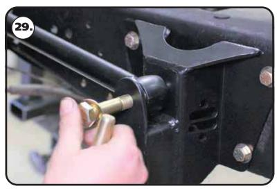
**29.** Line the through hole of the R-Joint with the of holes of the frame mount. Install a 5/8" flat washer on to a 5/8"-18 x 3 1/2" hex bolt, insert into the lined up holes. Install a 5/8" flat washer followed by a 5/8"-18 nylok nut. Repeat on both sides and tighten the bolts/nuts enough to eliminate any gaps.
