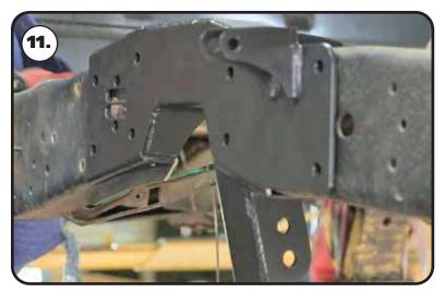
**11.** After cutting, slip the c-notch over the frame to check the fitment. The cut areas of the frame may require grinding for the c-notch to fit.
