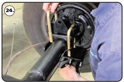
**24.** Install a supplied 5/8" u-bolt in each side of the upper bar mount. The u-bolts will nest in the slots of the upper mount. The U-bolts will run parallel to the axle tube.
