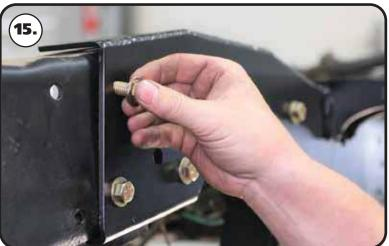
**15.** Install a 7/16" flat washer on each of (8) 7/16" x 1 1/4" bolts. This hardware gets installed in the sides of the c-notch. Install a 7/16" flat washer and 7/16" nylok nut on each bolt sticking through the frame. Tighten all of the c-notch side bolts. Tighten the hardware snuggly for the time being.
