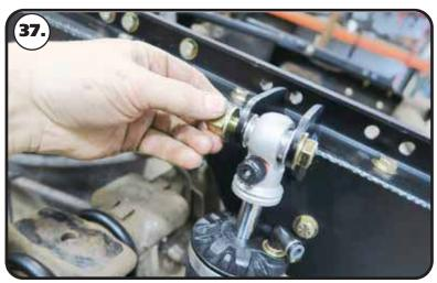
**37.** Insert the 1/2" ID Shock Bearing Spacers into the Bearing of the ShockWave/CoilOver. Install a 1/2" Flat Washer on a 1/2"-13 x 2 3/4" Bolts. Insert the top of the shock into the shock mount on the c-notch with the adjusting knob to the outside. Line up the holes and insert the bolt/washer. Install a 1/2" Flat Washer and 1/2"-13 Nylok Nut on the threads and tighten to 50 ftlbs.
