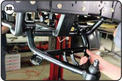
**38.** Insert the lower control arm in the mounts built in the lower cradle. Align the mounting holes of the lower mounts with the through hole of the bushing sleeves.
