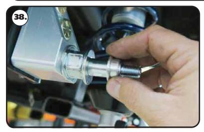
**38.** The Shock Stud requires spacers that are .400" long (90002067). Install a 5/8" ID 90002067 spacer **(Small side towards shock body)** onto the lower Shock Stud. Slide the bottom of the Shock onto the Stud. Install a second 5/8" ID 90002067 Spacer onto the Stud **(small side towards shock)**. You may need to jack the rear end up to Slide the Shock onto the Stud.
