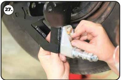
27. Insert the bolts through the axle mount and install the flat washers & nylok nuts on the threads sticking through. Repeat on both sides and torque the bolts/nuts to 75 ftlbs. Install a 5/8" flat washer onto the 5/8"-18 threads of the shock stud. Apply Red Loctite to the 5/8" threads of the stud. Thread the shock stud into the threaded hole of the lower mount. Repeat on both sides and torque the shock stud to 65-75 ftlbs.
