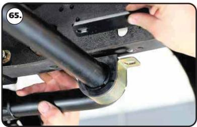
**65.** The sway bar includes a backer plate that needs to be installed on the top side of the frame flange. Align the backer plate holes with the holes drilled in the frame.
