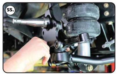
**55.** Install The steering arms on the spindles. The steering arms bolt to the bottom 2 holes of the spindle. The steering arms angle toward the rack, and the tie rod mounting holes are to the front of the truck. The steering arm attaching hardware is supplied with the spindle.
