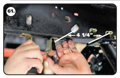
**61.** Use a tape measure to put a mark on the frame **4 1/4"** from the front edge of the cradle mount. Align the back edge of the sway bar mounting strap with the mark on the frame. Hold the mounting strap in the center of the frame and mark the center of each mounting hole. The mounting holes need to be marked on each frame rail.
