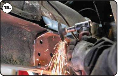
**15.** We grind the top of the cross member back to the frame rail.
