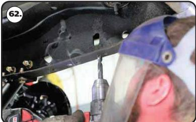
**62.** Drill the holes using a 3/8" drill bit.
