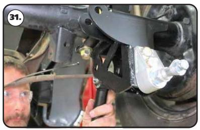
**31.** Insert (2) .625" ID x .740" long R-Joint spacers into the R-Joint of one end of each lower bar (23 1/8"). The small diameter of the spacer goes into the R-joint. Insert the rear lower bar R-Joint into the lower bar mount built into the axle mount.
