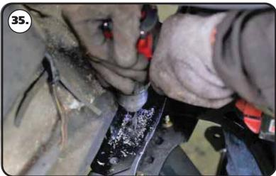
**35.** The top flange of the upper control arm mount has (4) mounting holes. (2) of these mounting holes will align with OEM holes. (2) need to be drilled with a 7/16" drill bit.
