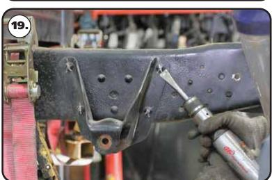
19. The OEM front leaf spring mounts will need to be removed from the frame rail. This can be done by either drilling the rivets out or removing the rivet heads and driving them out. We remove the rivet heads by cutting a "+" in the head with a die grinder then we cut the head off with a hammer and chisel or with an air chisel.
