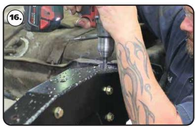
**16.** Use a 7/16" drill bit to drill the remaining holes in the top and bottom of the frame.
