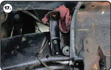
**17.** Your truck may have a brake line bracket right behind the coil spring mount that will need to be removed from the frame rail. This mount usually attaches with a rivet and bolt. Remove the bolt and rivet to remove the mount.
