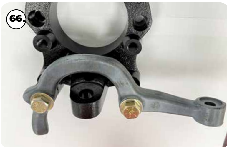
66. Hold the steering arm slugs in place. Align the mounting holes of the steering arm with the threaded holes of the slugs. Driver side steering arm is shown in Image 66 . The tie rod end curves in to the inside of the truck. Install a 1/2" flat washer on a 1/2"-13 x 2" & 1/2"-13 x 2 1/4" hex bolts. The 1/2"-13 x 2 1/4" bolt will go in the hole closest to the tie rod end. Apply red loctite to the threads of the bolts before threading into the slugs. It is the thicker side of the mounts. Insert a bolt in each steering arm hole and thread them into the steering arm slugs. Torque to 80 ft-lbs. Repeat on other steering arm/spindle. Make sure the end of the bolt is sticking out of the slug.
